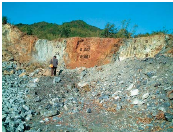
図3-9 相谷採石場北斜面にて 数値は帯磁率(SI) Fig. 3-9 At north site of Aitani quarry. Attached numbers are susceptibility value (SI unit).
