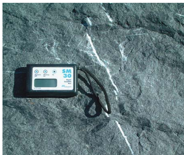
図3-8 帯磁率計 Fig. 3-8 Handy susceptibility meter
