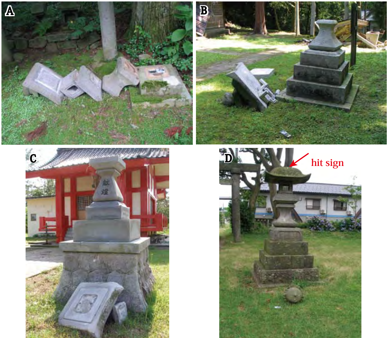
FIGURE 5. Field occurrences of fallen-down joyato-type stone lanterns. A, Fall-down of lower column; B, Fall-down of middle platform; C, Fall-down of light box. D, Fall-down of orb, which is an uppermost part of an joyato-type stone lantern. Red arrow shows the hit sign.
