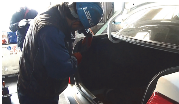
Fig. 5 Dismantlement Test 2 of Rear Bumper of Mazda Familia (Remove Endplate Trim)
