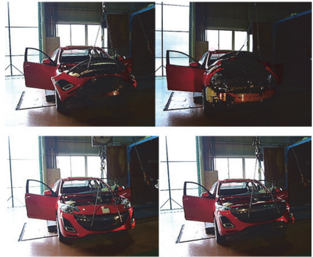
Fig. 9 Dismantlement Test of Bumper Designed for Recycling
