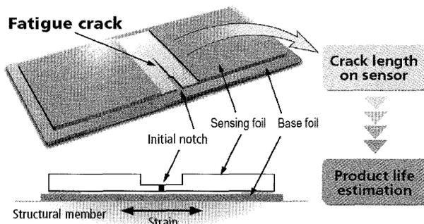
Figure 5 Construction of FDS
