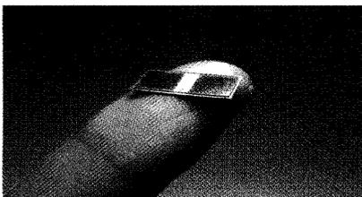
Figure 3 Fatigue Damage Sensor (FDS)
