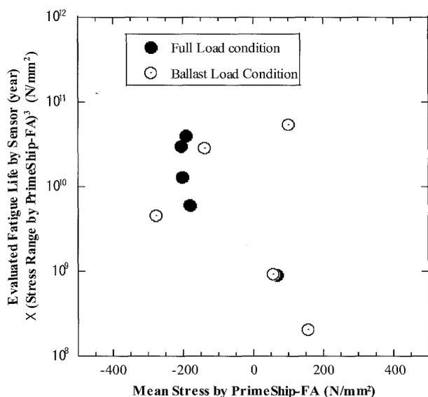
Figure 10 Sensor's Sensitivity to Mean Stress
