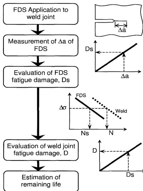
Figure 6 Flow of Fatigue Life Evaluation Using FDS
