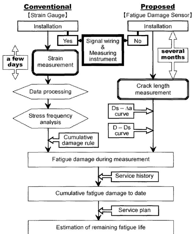
Figure 4 Comparison of fatigue remaining life estimation methods using strain gauge and FDS
