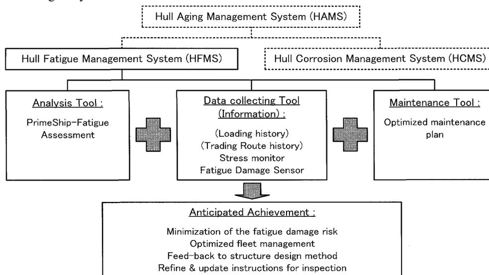
Figure 1 Schematic Diagram of Hull Fatigue Management System (HFMS)
