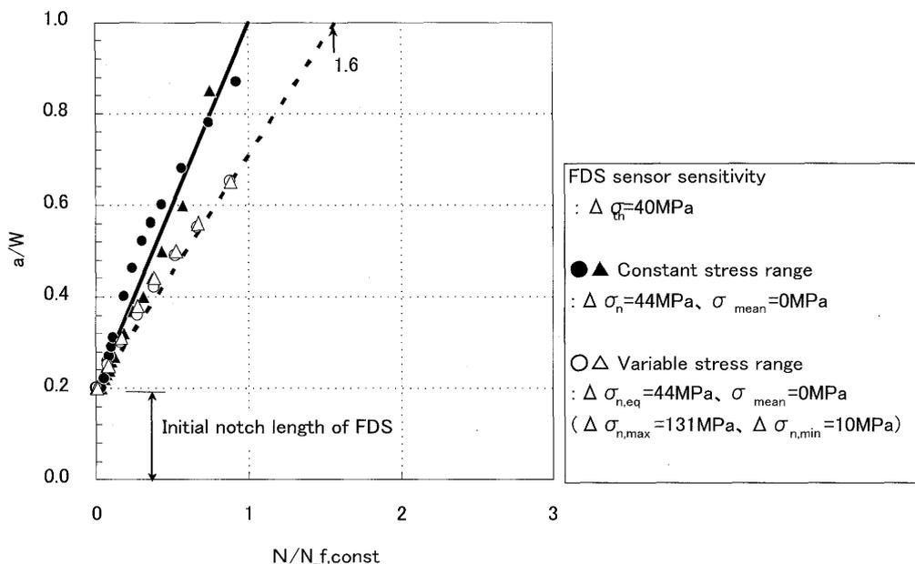
Figure 8 Crack propagation characteristics of FDS (Case 1)
