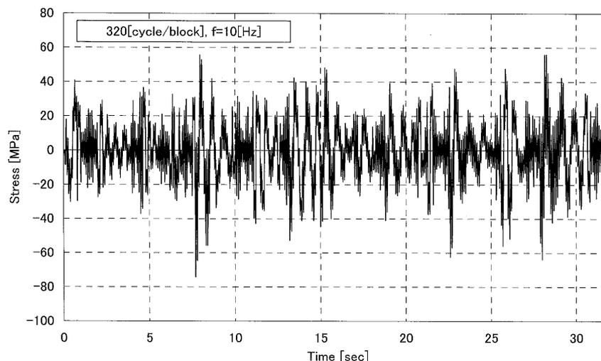
Figure 7 Input Stress Wave of Variable Stress range Test (Case-1)
