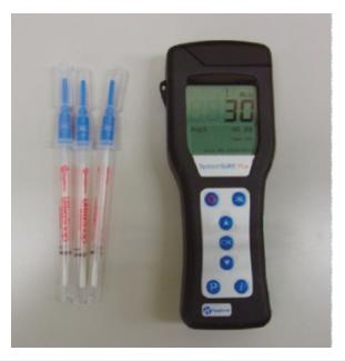
An ATP test kit and equipment. Adenosine triphosphate (ATP) is a molecule found in living cells and as such can be used to inspect for the growth of microorganisms such as bacteria and mold.
