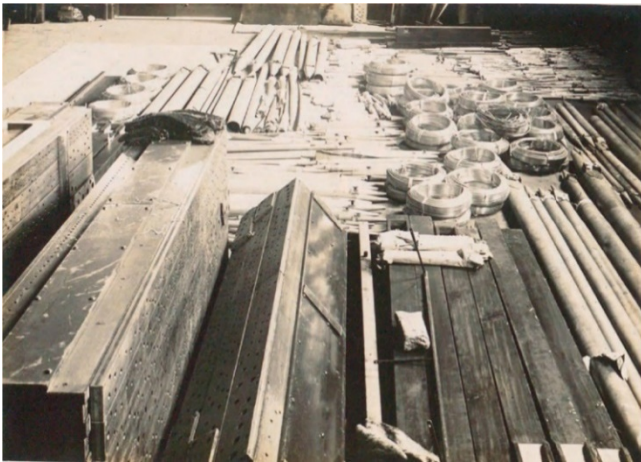
Parts of the pipe organ laid out on the floor. Shown in the background of the image are metal pipes and wound lead conductors. In the left foreground are windchests and on the right are wooden pipes. Approximately 1,400 pipes were used for the pipe organ built in the Nanki Concert Hall.
