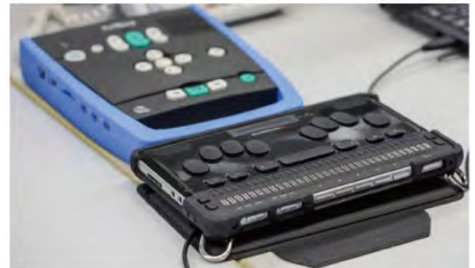
A device for text-to-speech with braille display (front) and a DAISY data player (back).
