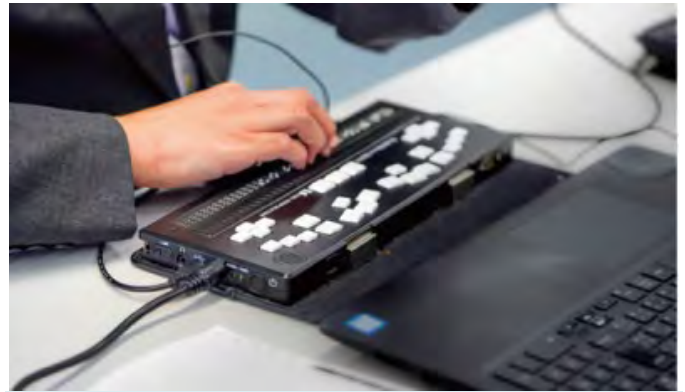
The text on the screen can be read by touching this braille display.
