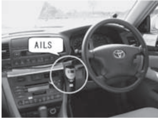
Fig. 1 Condition of installing the AILS (Passenger car)
