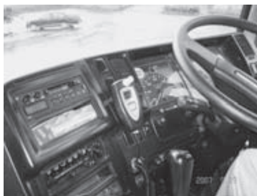
Fig. 2 AILS Installed in a Commercial Truck
