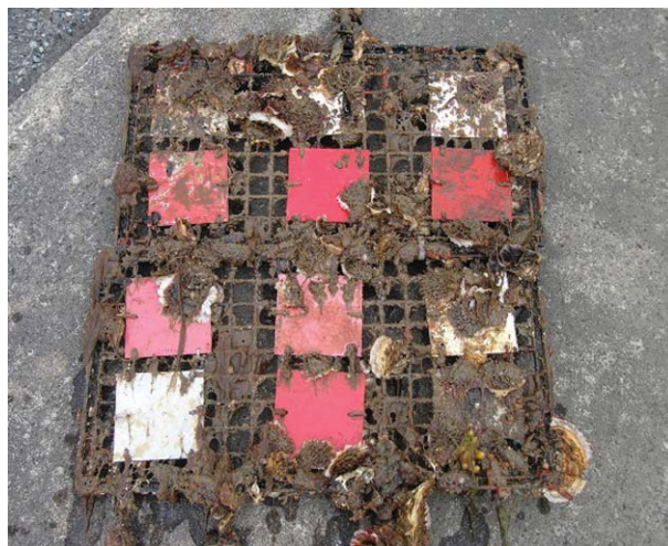
Fig. 2. Results of antifouling tests. See Table 1 for antifouling paints used. The plate-1 is the control (aluminum plate only) without antifouling paint.
