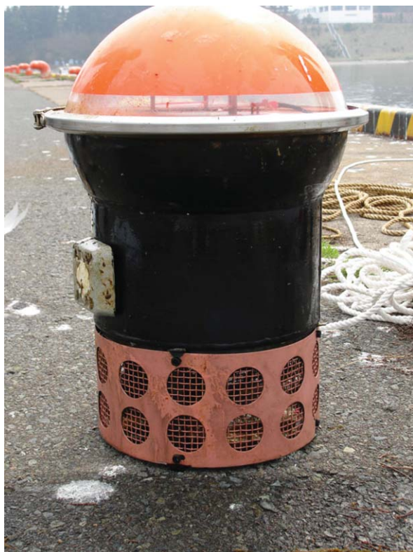
Fig. 3. Drifting buoy system with sea surface pCO 2 sensor. The silicon-based antifouling paint (CMP Bioclean C, clear and colorless) was used as biofouling prevention for the surface (black portion) of our drifting buoy system. The black color of the surface is from the epoxy resin paint (under coat).
