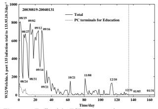
Figure 3. Traffic of the TCP port 135 infection access to the IP address of 133.95.10.3 through August 19th, 2003 to January 31st, 2004 (day<sup>-1</sup> unit). Both solid and dotted lines show the total traffic and the traffic from PC terminals for education (133.95.3x.0/24), respectively.
