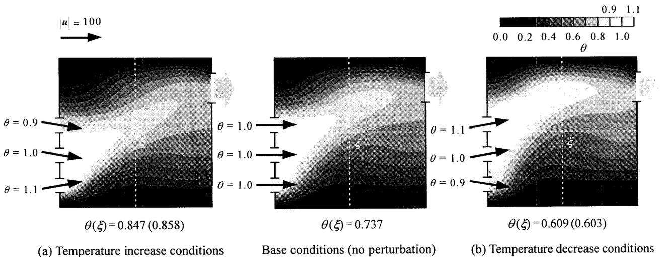
Fig. 6 Thermal and flow inlet conditions to increase and decrease temperature at  $\xi$
