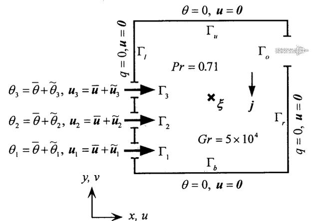
Fig. 4 Configuration of mixed convection heat transfer in a square cavity ( $\bar{\theta} = 1, \bar{u} = (100, 0)^T$ )
