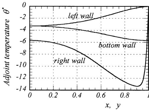
Fig. 3 Influence of wall heat flux distributions on temperature at the center of cavity
