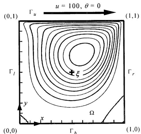
Fig. 1 Configuration of forced convection heat transfer in a square cavity
