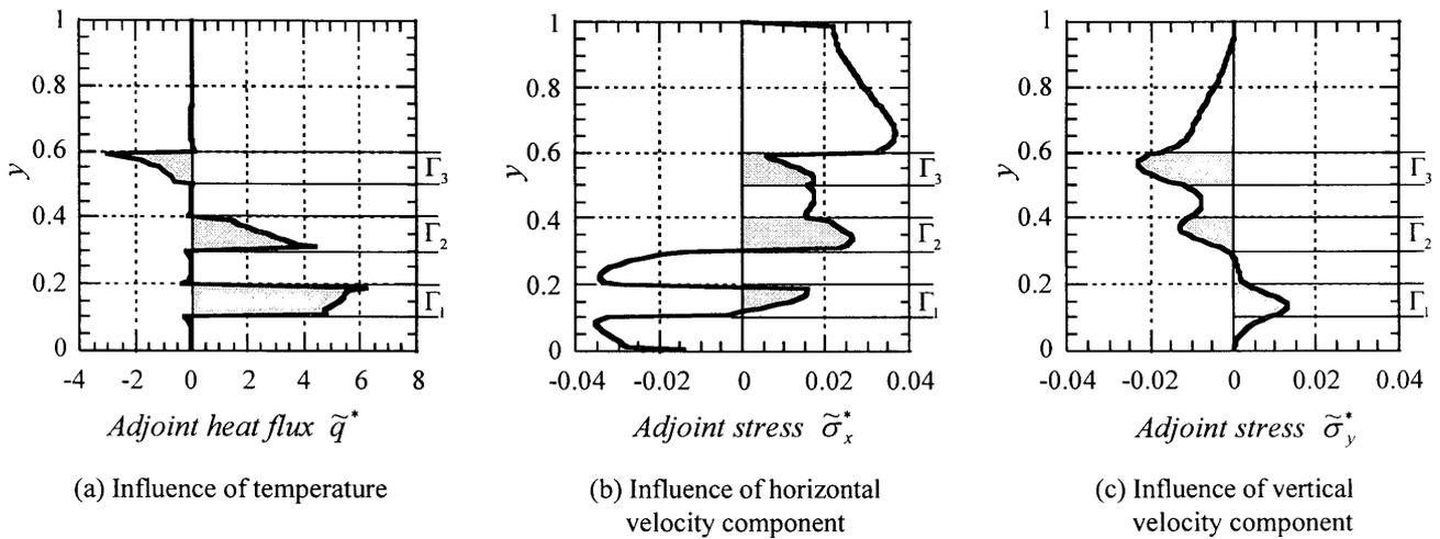
Fig. 5 Influences of thermal and flow perturbations at inlets on temperature at the center of cavity
