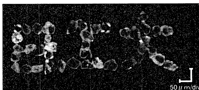
Fig.5 Diamond grains arranged using the micromanipulator
