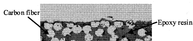
Fig.6 Micrograph of CFRP surface
