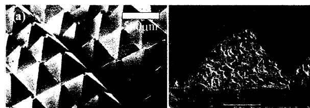
Fig. 1 SEM image of pyramidal structure polishing pad
