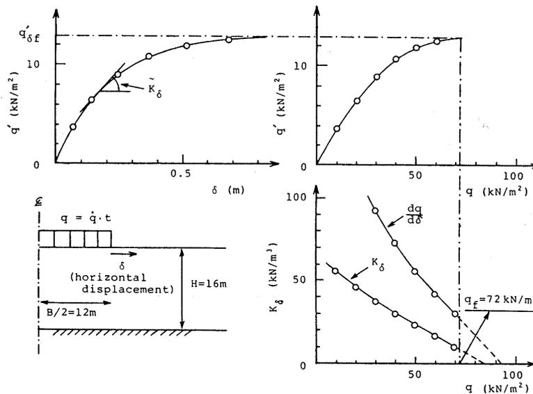
Fig. 10. Prediction procedure for bearing capacity of saturated soil deposit (Asaoka and Ohtsuka, 1986)
