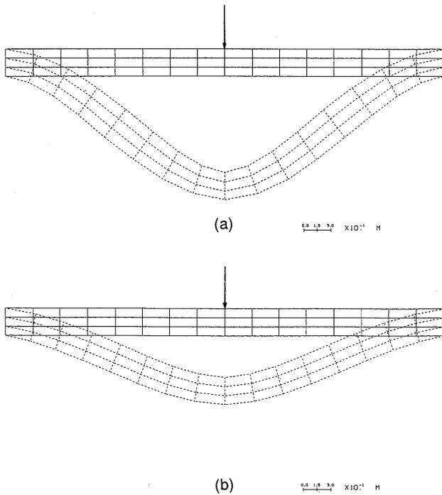
Fig. 9. Deformed profile for simple beam
