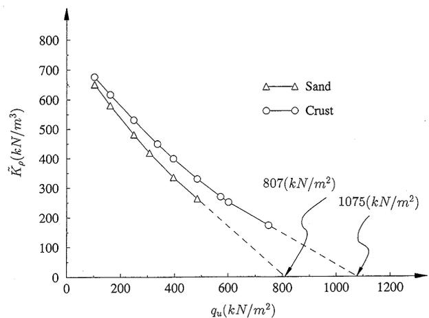
**Fig. 13. Deterioration of tangential stiffness factors**
