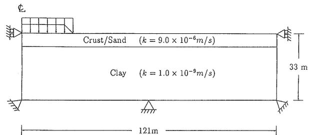
Fig. 11. Two-layered soil deposit
