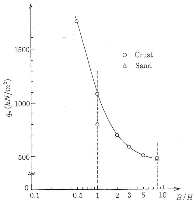
**Fig. 14. Estimated bearing capacity**
