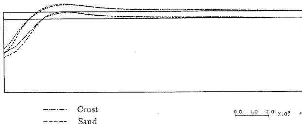
**Fig. 12. Deformation profiles based on different modeling of surface layer**
