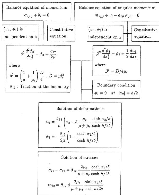
Fig. 6. Solution procedure
