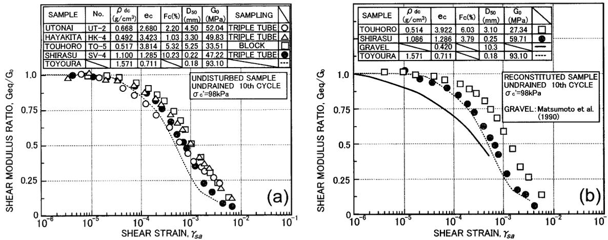
Fig. 11. Relationships between  $G/G_0$  and  $\gamma_{sa}$ : (a) undisturbed samples and (b) reconstituted samples
