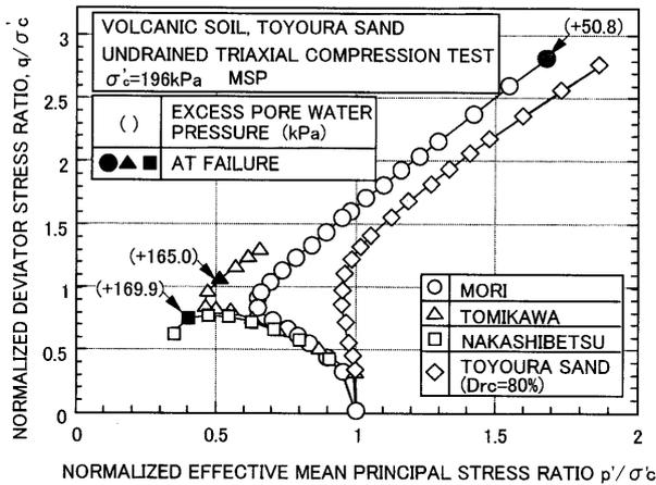
Fig. 5. Undrained effective stress paths for volcanic soils and Toyoura sand ( $\sigma'_c = 196$  kPa)
