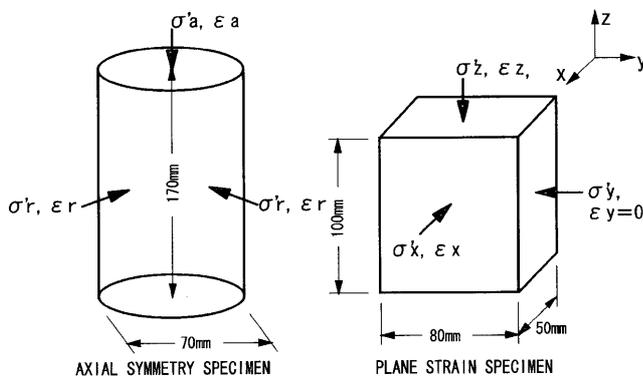
Fig. 3. Dimension of the specimen and stress and strain parameters
