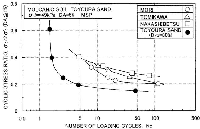
Fig. 8. Liquefaction strength for volcanic soils and Toyoura sand
