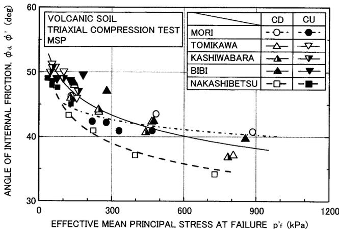
Fig. 6. Dependency of  $\phi_d$  and  $\phi'$  on effective mean principal stress
