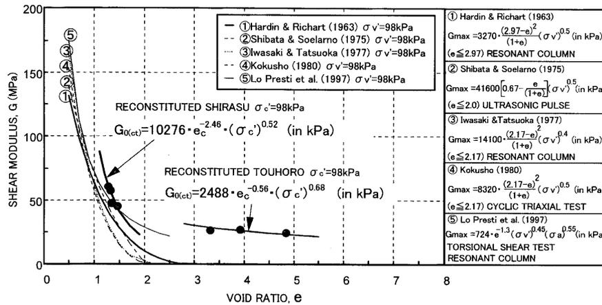
Fig. 14. Small strain shear modulus  $G$  related to void ratio
