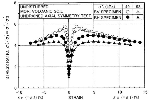
Fig. 9. Effect of fabric anisotropy on static stress-strain behavior for undisturbed Mori volcanic soil
