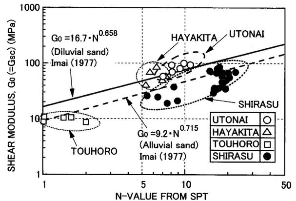
Fig. 15. Relationships between shear modulus  $G_0 (= G_{sc})$  and  $N$  value from SPT
