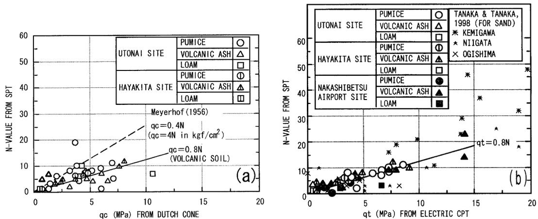
Fig. 16. Relationships between  $N$  value and cone penetration test results: (a)  $q_c$  vs.  $N$  and (b)  $q_t$  vs.  $N$
