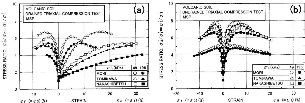
Fig. 4. Comparisons of stress-strain relationships: (a) drained triaxial compression tests and (b) undrained triaxial compression tests
