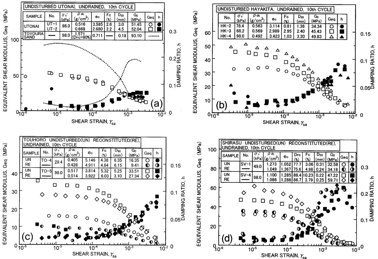
Fig. 10. Cyclic deformation properties for undisturbed (UN) and reconstituted (RE) volcanic soils: (a) Utonai, (b) Hayakita, (c) Touhoro and (d) Shirasu
