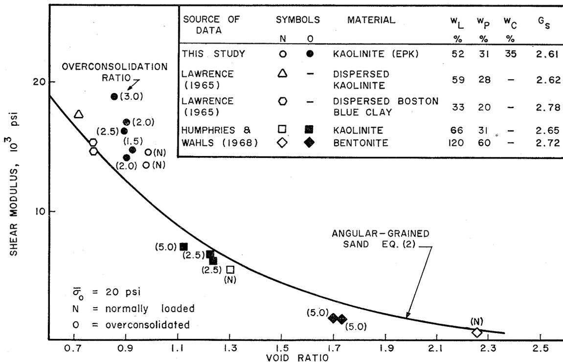
Fig. 14. Effect of overconsolidation ratio on shear modulus of saturated clays
