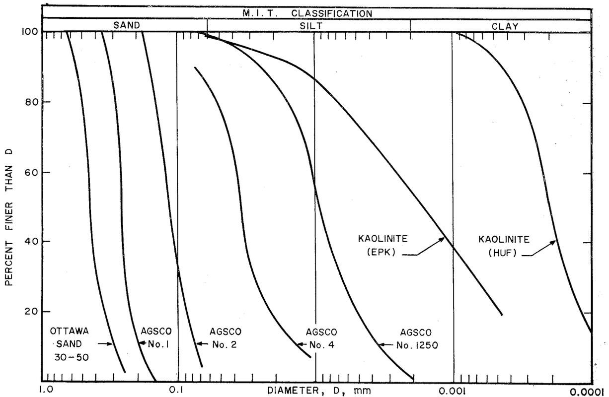
Fig. 2. Grain size distribution curves
