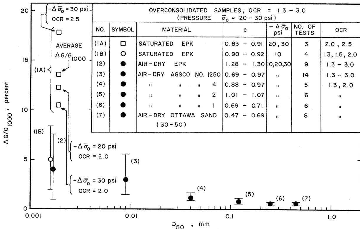
Fig. 10. Summary diagram illustrating ranges and average values of time-dependent modulus increase for different soils—overconsolidated condition
