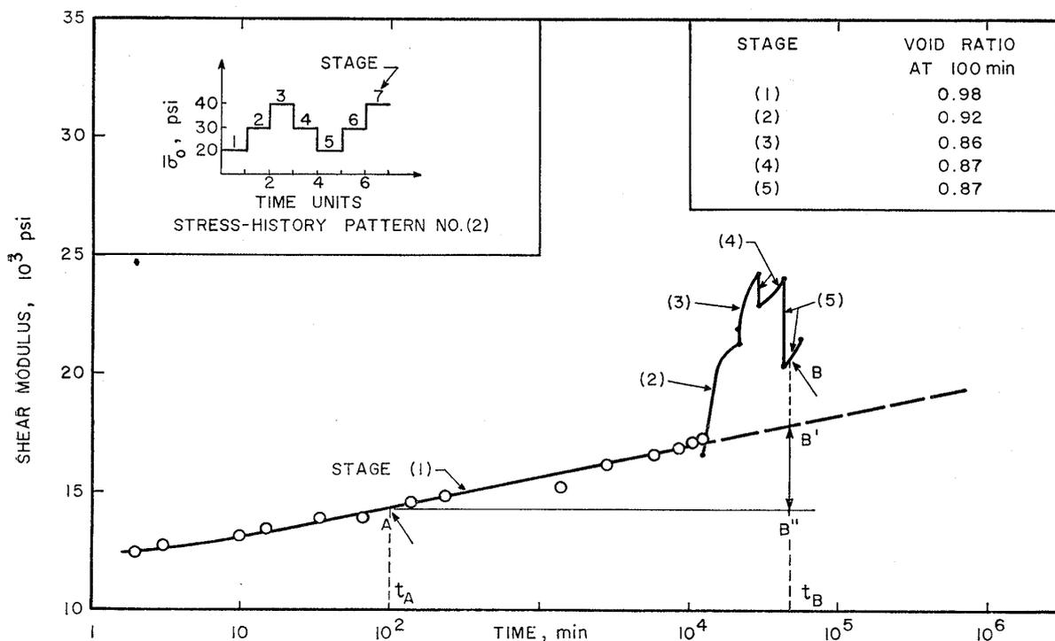
Fig. 12. Method of separating effects of overconsolidation ratio and time between stages (1) and (5) of stress-history pattern No. 2
