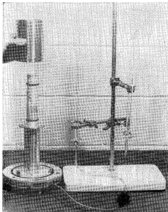
**Photo. 2. Installation of fluid jacket cylinder around a sample of saturated clay**
