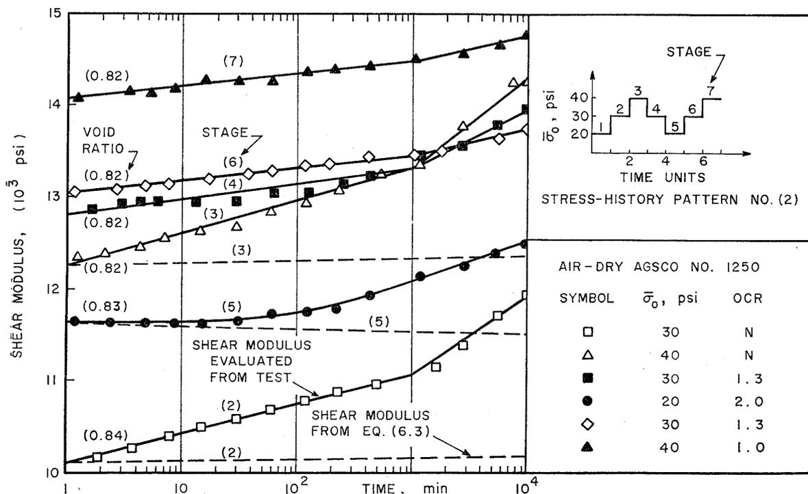
Fig. 11. Variation of shear modulus with time and confining pressure for air-dry crushed-quartz silt
