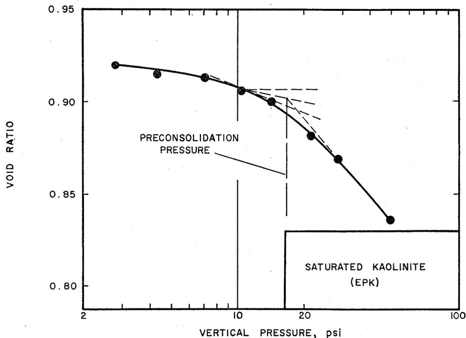
Fig. 4. Void ratio vs. pressure for saturated kaolinite clay
