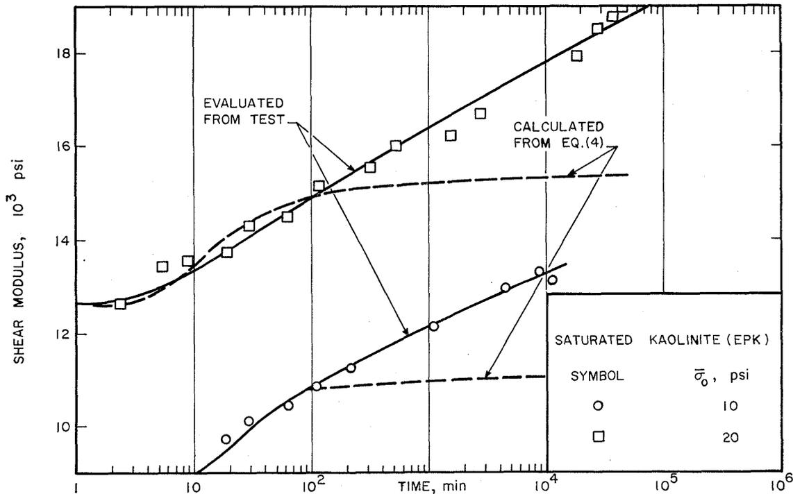
Fig. 8. Variation of shear modulus with time for saturated kaolinite clay
