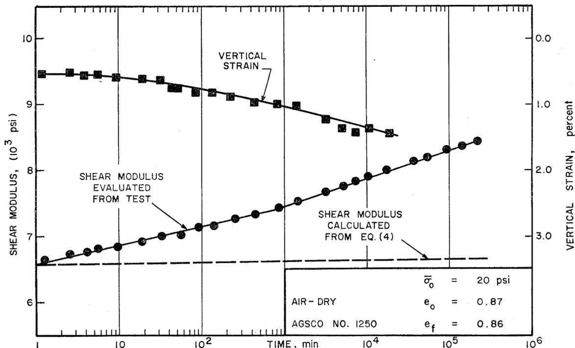
Fig. 5. Variation in shear modulus and vertical strain with time for a sample of air-dry crushed-quartz silt subjected to constant confining pressure
