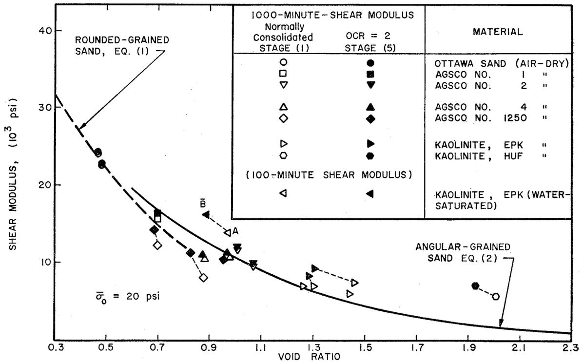
Fig. 13. Comparison between results of stages (1) and (5) of stress-history pattern No. 2 after accounting for effects of time
