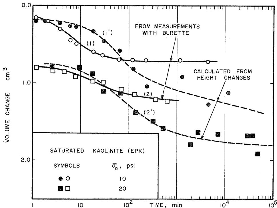
Fig. 6. Comparison between measured and calculated changes in volume with time for a sample of water-saturated clay subjected to constant confining pressures
