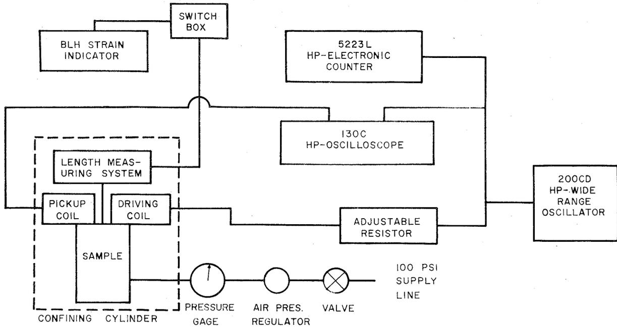
Fig. 1. A schematic diagram of the test setup
