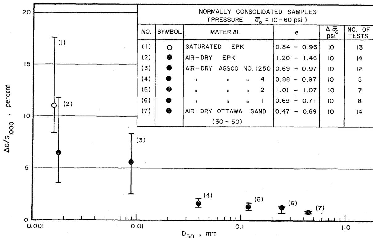
Fig. 9. Summary diagram illustrating ranges and average values of time-dependent modulus increase for different soils—normally consolidated condition
