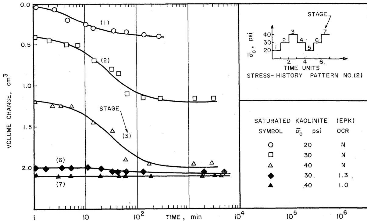
Fig. 7. Variation of volume with time and confining pressure for water-saturated kaolinite clay
