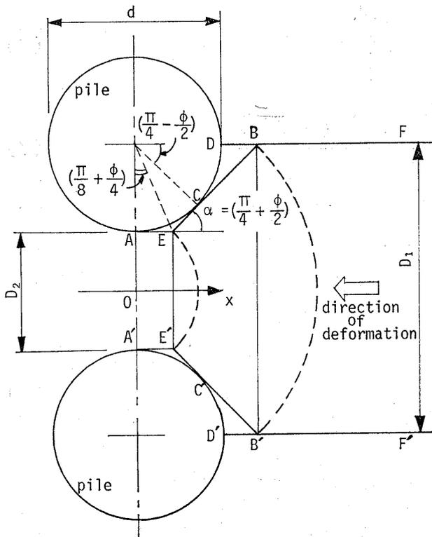
Fig. 2. State of plastic deformation in the ground just around piles
