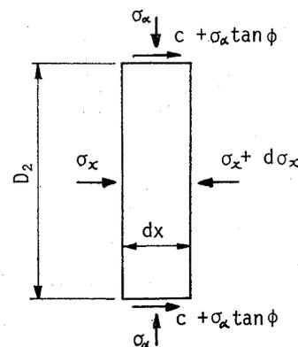
Fig. 4. Small element of plastically deforming ground (AEE'A')
