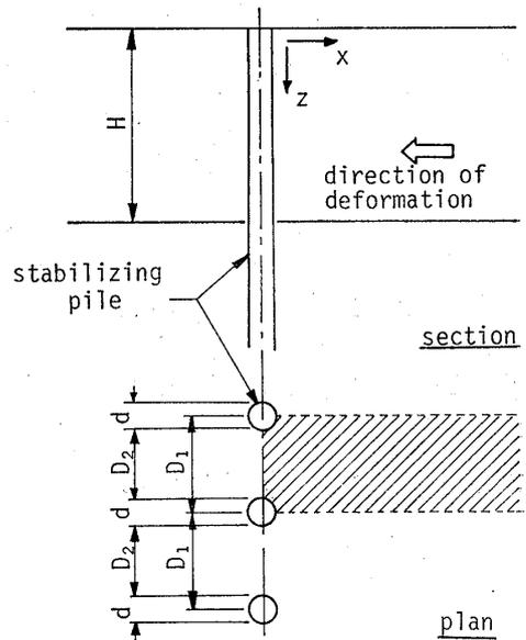
Fig. 1. Stabilizing piles in a row through plastically deforming ground
