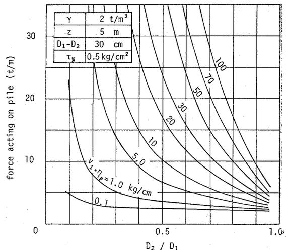
Fig. 10. The effect of product of flow velocity and plastic viscosity ( $v_1 \cdot \eta_p$ ) on the theory of plastic flow
