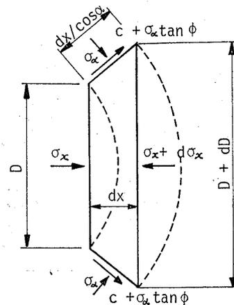
Fig. 3. Small element of plastically deforming ground (EBB'E')
