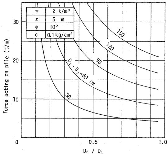
Fig. 9. The effect of pile diameter ( $D_1 - D_2$ ) on the theory of plastic deformation
