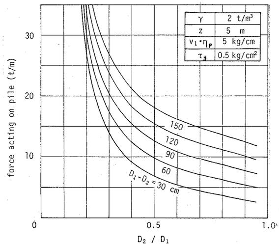
Fig. 12. The effect of pile diameter ( $D_1 - D_2$ ) on the theory of plastic flow
