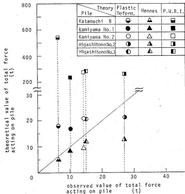
Fig. 14. Comparison between the theoretical and the observed values of total lateral force acting on stabilizing piles against landslides
