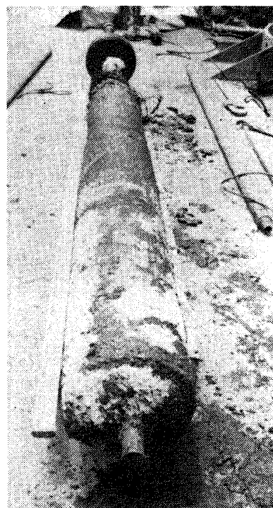
Photo. 2. The frozen soil column obtained at site B
