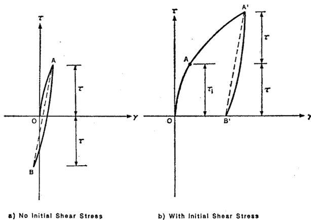
Fig. 8. Conventional interpretation of shear modulus in cyclic loading tests (schematic)
