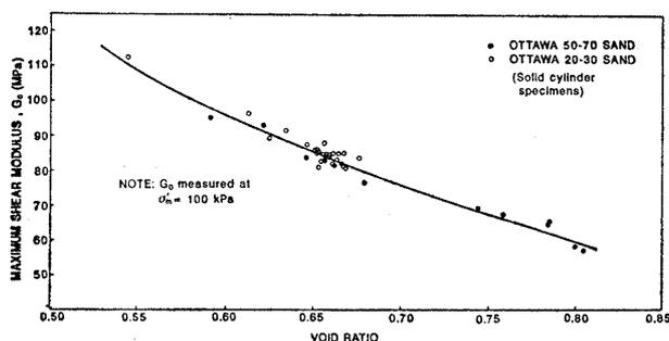
Fig. 3. Variation of maximum shear modulus with void ratio
