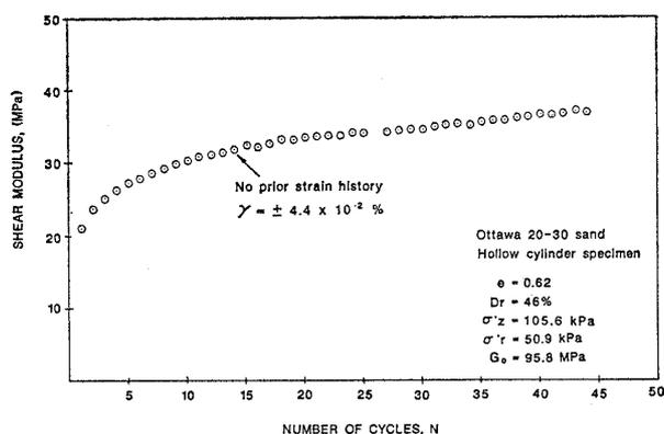
Fig. 14. Variation of shear modulus with number of cycles
