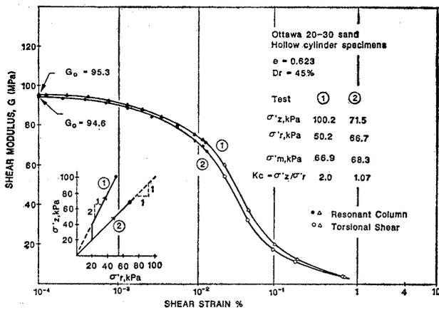
Fig. 7. Effect of consolidation stress ratio on modulus reduction curve
