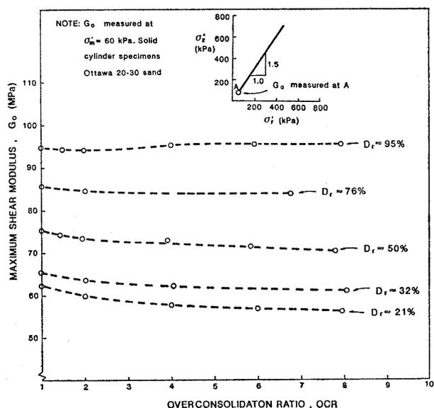
Fig. 11. Effect of axial compression pre-stressing on maximum shear modulus
