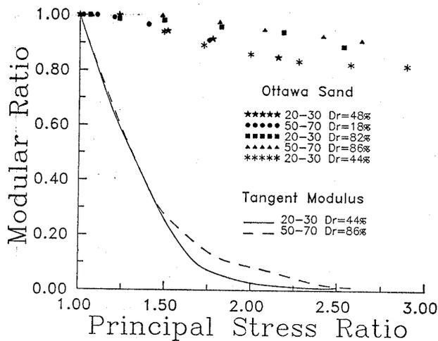
Fig. 6. Effect of principal stress ratio on modular ratio
