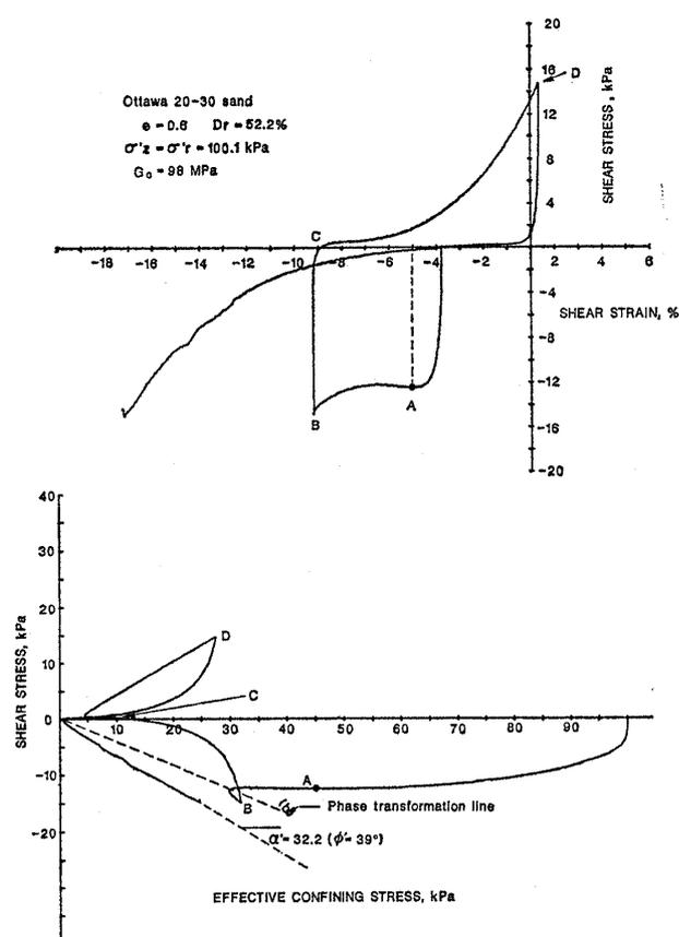
Fig. 16. Cyclic torsional shear test-reconsolidated specimen
