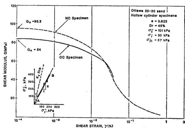
Fig. 10. Effect of axial compression prestressing on modulus reduction curve
