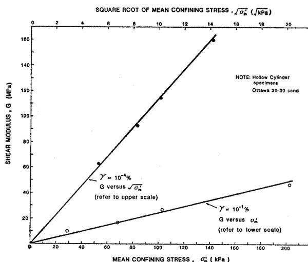
Fig. 5. Relationship between shear modulus and mean confining stress
