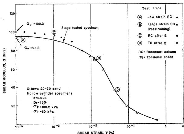
Fig. 12. Effect of cyclic prestraining on modulus reduction curve
