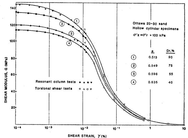
Fig. 1. Effect of relative density on shear modulus-shear strain relationship
