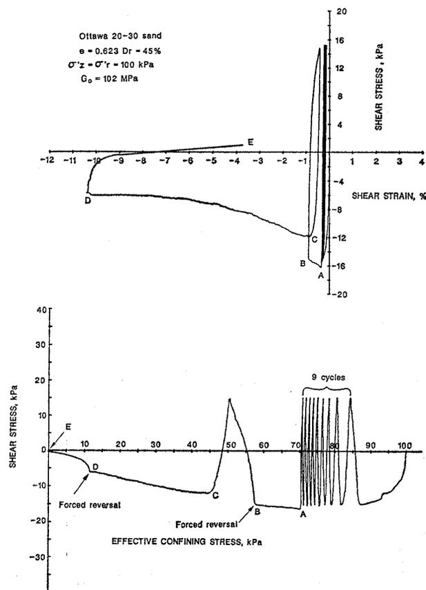
Fig. 15. Cyclic torsional shear test-virgin specimen
