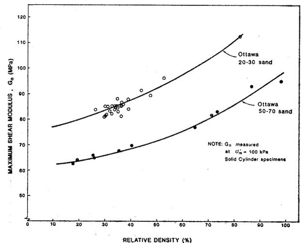
Fig. 2. Variation of maximum shear modulus with relative density
