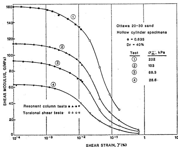
Fig. 4. Effect of confining pressure on shear modulus-shear strain relationship
