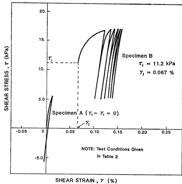
Fig. 9. Influence of initial stress conditions on the undrained cyclic shear stress-shear strain relationship
