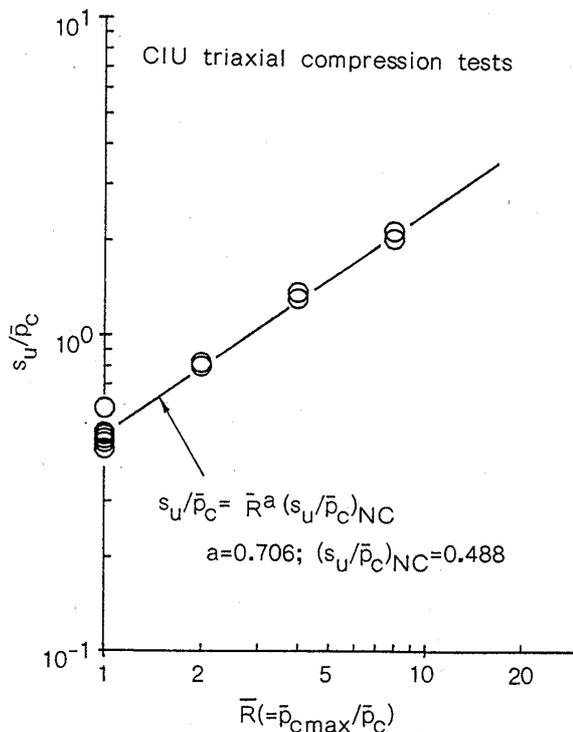
Fig. 11. The relationships between the ratio of the triaxial undrained strength,  $s_u$ , to the consolidation pressure,  $\bar{p}_c$ , and the overconsolidation ratio  $R$ . Results from CIU triaxial tests
