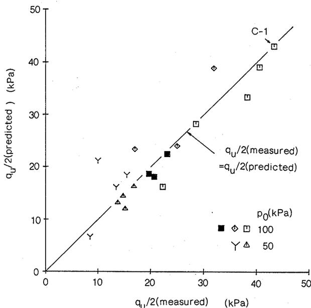
Fig. 10. The comparison of unconfined compressive strengths predicted by  $A_f - \bar{R}$  relationship obtained from triaxial tests with measured ones
