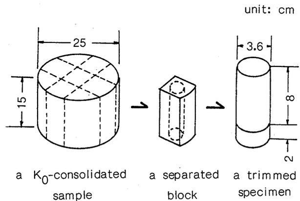
Fig. 1. Procedure for preparing specimens for unconfined compression tests
