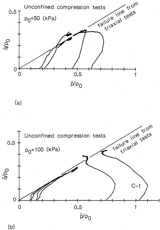
Fig. 8. Effective stress paths in unconfined compression tests: (a)  $p_0=50$  kPa; and (b)  $p_0=100$  kPa
