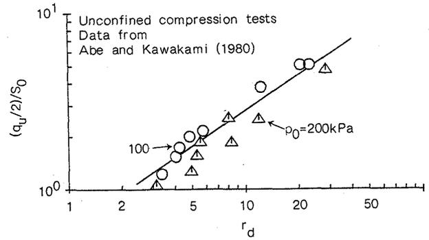
Fig. 13. The relationships between the ratio of the unconfined compressive strength,  $q_u/2$ , to the initial suction,  $S_0$ , and the disturbance ratio,  $r_d$ ; replotted from results in Abe and Kawakami (1980)
