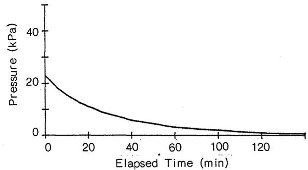
Fig. 3. The dissipation of the water pressure caused by closing the valve of the transducer
