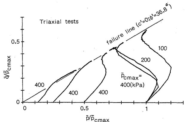
Fig. 6. Effective stress paths in CIU triaxial tests.
