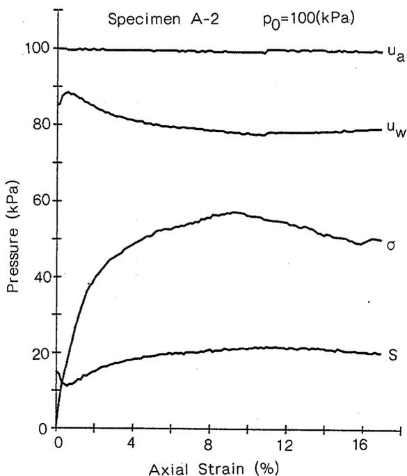
Fig. 7. Typical results of an unconfined compression test
