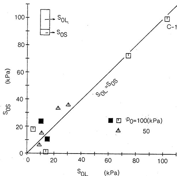
Fig. 14. The comparison of the initial suction measured for long specimens  $S_{OL}$  and short ones  $S_{OS}$
