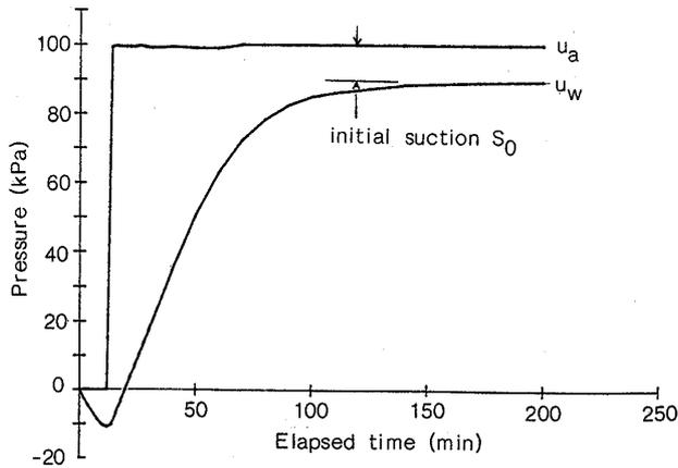
Fig. 4. An example of the variations of the air and water pressures with time. The constant value of the difference between them is the initial suction
