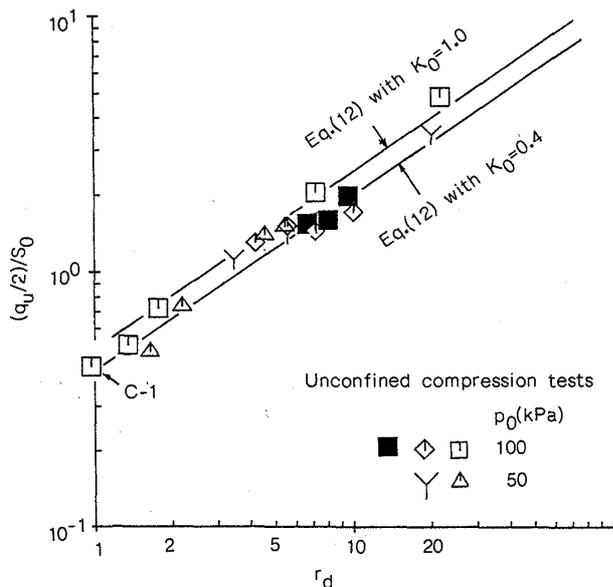
Fig. 12. The relationships between the ratio of the unconfined compressive strength,  $q_u/2$ , to the initial suction,  $S_0$ , and the disturbance ratio,  $r_d$ ; results from unconfined compression tests
