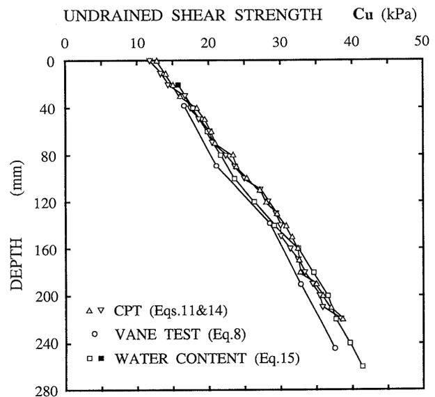
Fig. 13. Estimated undrained shear strength profile
