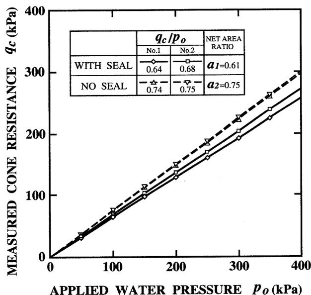
Fig. 4. Result of calibration test
