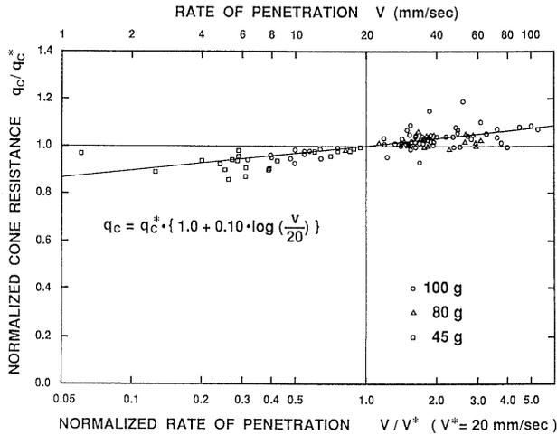
Fig. 11. Rate effect observed in CPT
