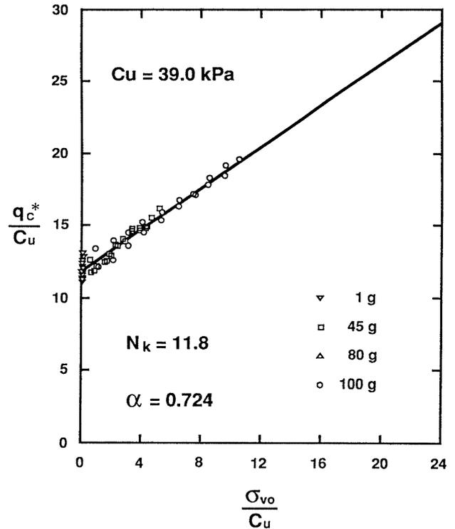
Fig. 12. Typical example of  $(q_c^*/c_u) \sim (\sigma_{vo}/c_u)$  relation (No. 2)
