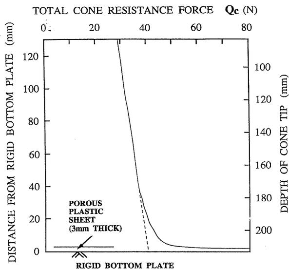
**Fig. 10. Analyzed  $Q_c$  data of the test in which the cone tip struck the bottom (No. 1, 80 g, hydraulic jack)**
