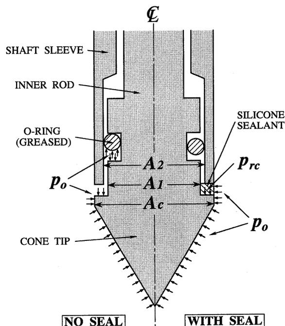
Fig. 5. Pressures around the cone tip
