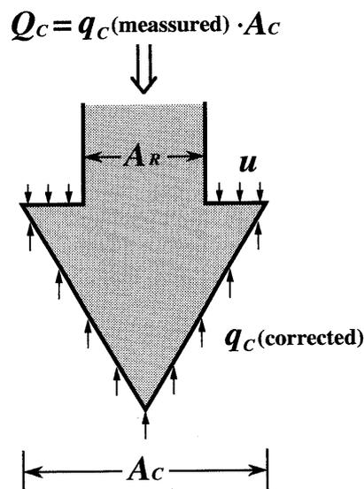
Fig. 1. Influence of pore water pressure behind the cone tip
