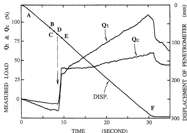
Fig. 7. Original time records of centrifuge CPT
