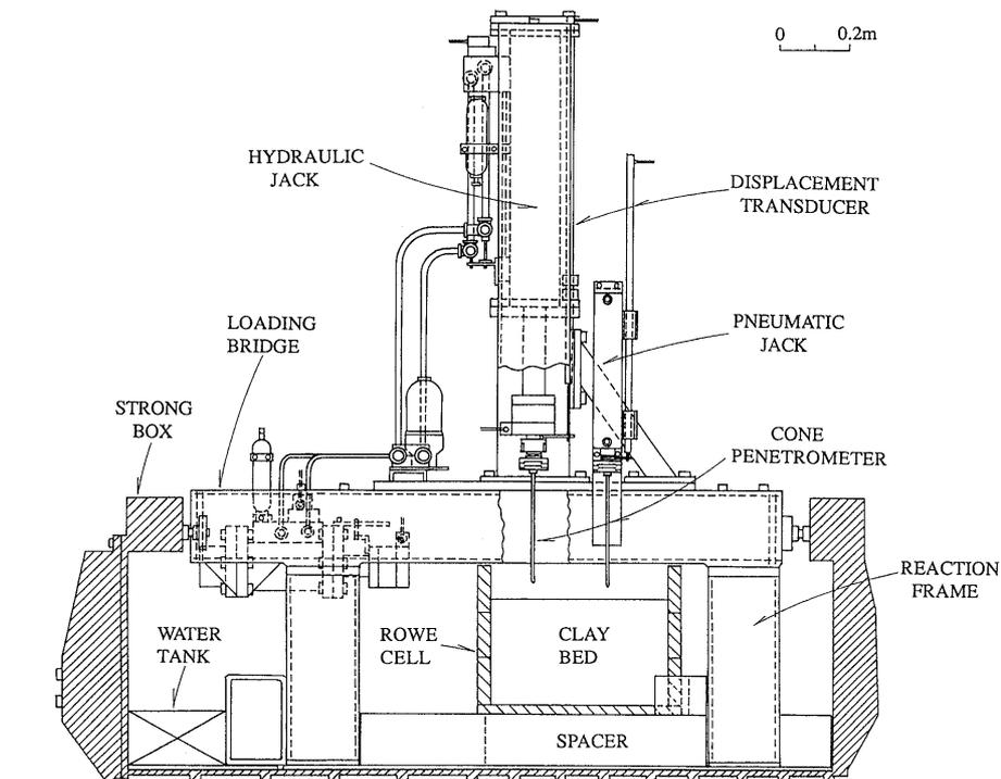
Fig. 6. Experimental setup in the centrifuge strong box
