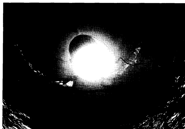
Fig. 7 Deposition of inner diameter of tubular structure using PBII & D technology. The tube size is about 5 cm in dia. \times 30 cm long.
