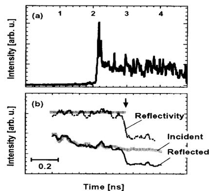
Fig. 4 (a) Typical temporal profile of the rear emission at a 40  $\mu\text{m}$ -thickness of Al. The drive laser irradiance is  $9.2 \times 10^{13} \text{ W/cm}^2$ . (b) Typical reflectivity signal, and the intensity profile of reflected and incident probe light to determine the reflectivity. Horizontal grey line shows 100% reflection. Shock arrival time is indicated by an arrow.
