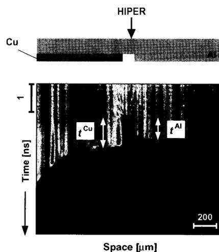
Fig. 5 Streaked image with double standard target by reflected light measurement. The step height of Al and Cu are 19.68 and 19.79  $\mu\text{m}$ , respectively. The  $t^{\text{Al}}$  and  $t^{\text{Cu}}$  indicate transit time for the shock traveling through each step, respectively.
