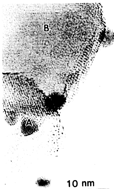
Fig. 6 High-resolution TEM images and X-ray spectra detected with EDS system, from catalyst particles (Au) distributed on TiO 2 substrate.
