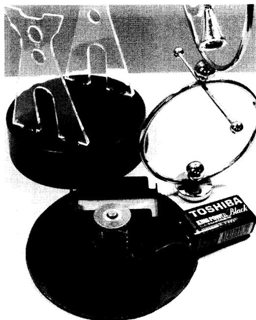
**Fig. 6** Internal mechanism of a swing toy. A search coil and a kick coil are wound around the same steel core. The search coil detects the magnet of the pendulum approaching. The induction electric current is amplified by a transistor. The kick coil is magnetized by an amplified current and repels the magnet of the pendulum.
