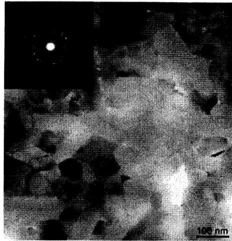
Fig. 10 TEM photograph and electron diffraction patterns of melt-spun  $\text{D}_{12.5}\text{Fe}_{69.8}\text{Co}_{10}\text{Nb}_1\text{Y}_{0.7}\text{B}_6$  alloy ribbons annealed at  $650^\circ\text{C}$  for 10 min.
