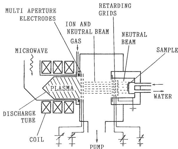
Fig. 1. Magneto-microwave plasma apparatus for ion and neutral beam irradiation.
