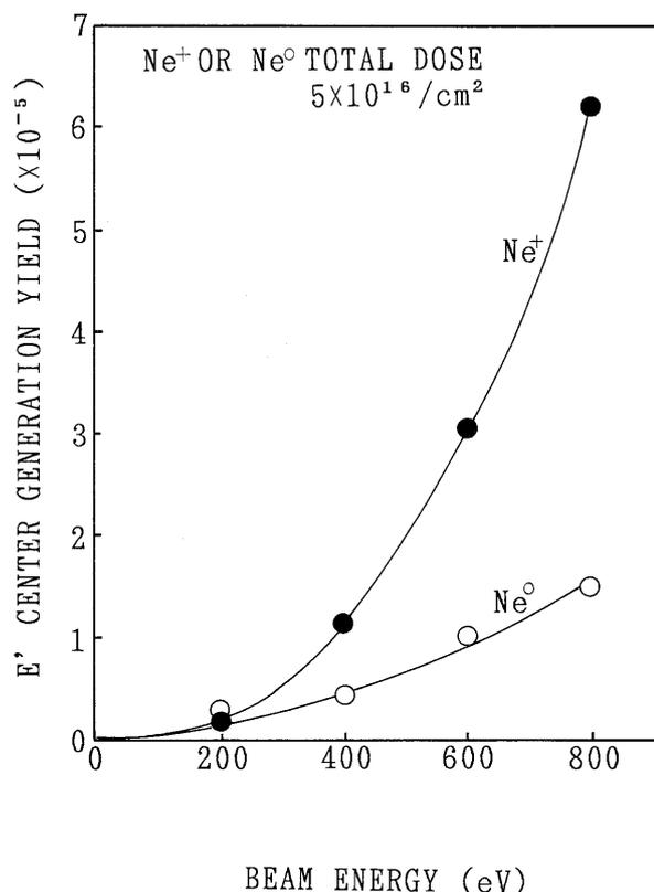
Fig. 4.  $E'$  center generation yield as a function of the kinetic energy of  $Ne^+$  and  $Ne^0$  beams.
