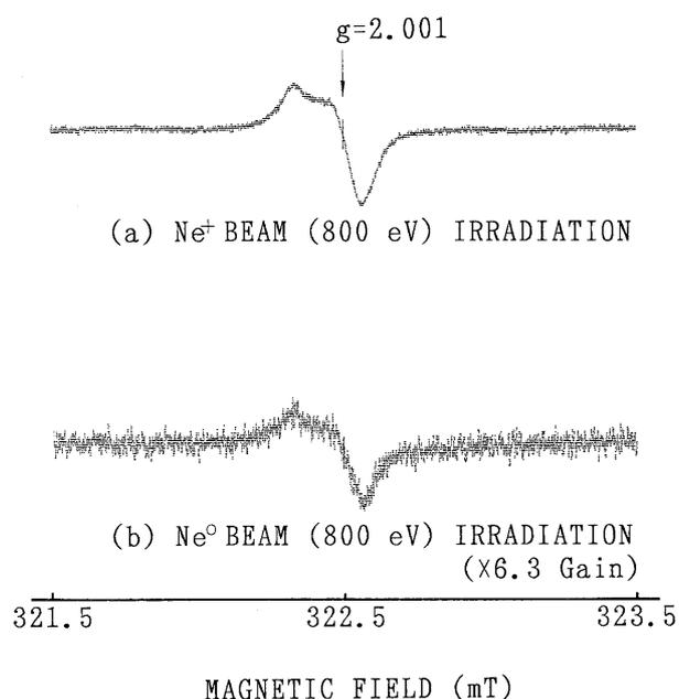
Fig. 2. ESR spectra of  $SiO_2/Si$  samples after (a)  $Ne^+$  beam, and (b)  $Ne^0$  beam irradiation.
