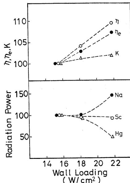
Fig. 4 Radiation properties as a function of the specific wall loading.
