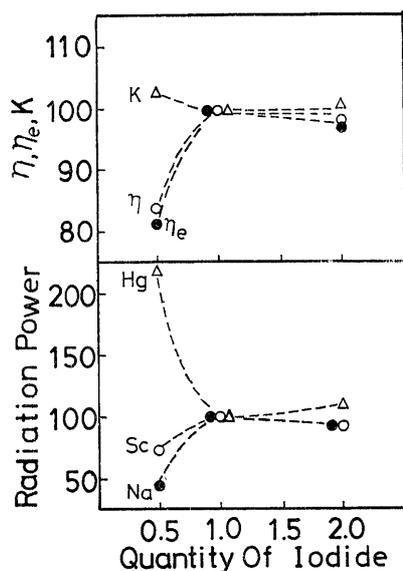
Fig. 2 Radiation properties as a function of the relative quantity of iodides.
