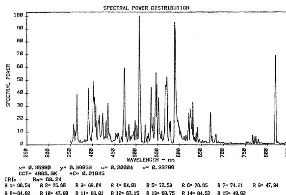
Fig. 9 The spectral power distribution of the newly designed 400W lamp.
