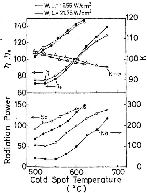
Fig. 6 Radiation properties with different inner diameters as a function of the cold spot temperature.
