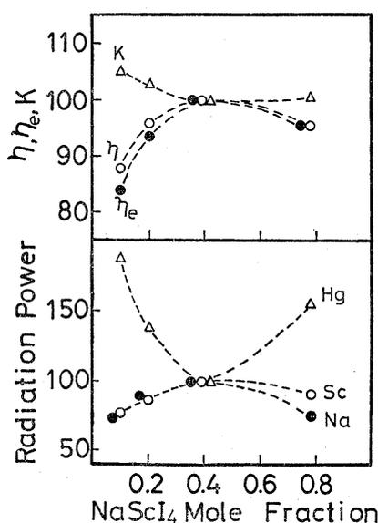
**Fig. 1** Radiation properties as a function of NaScI<sub>4</sub> mole fraction.
