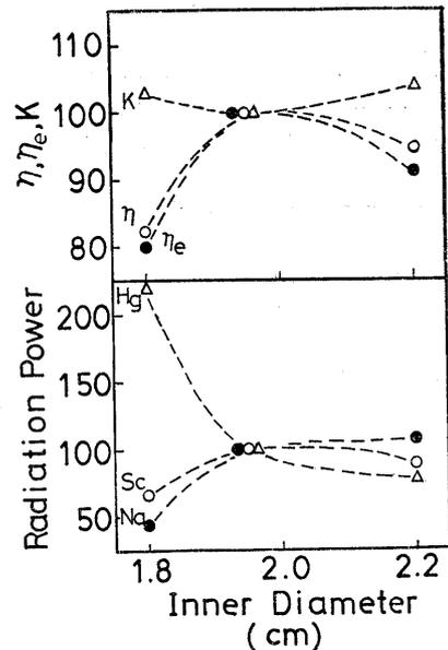
Fig. 3 Radiation properties as a function of inner diameter of the arc tube.
