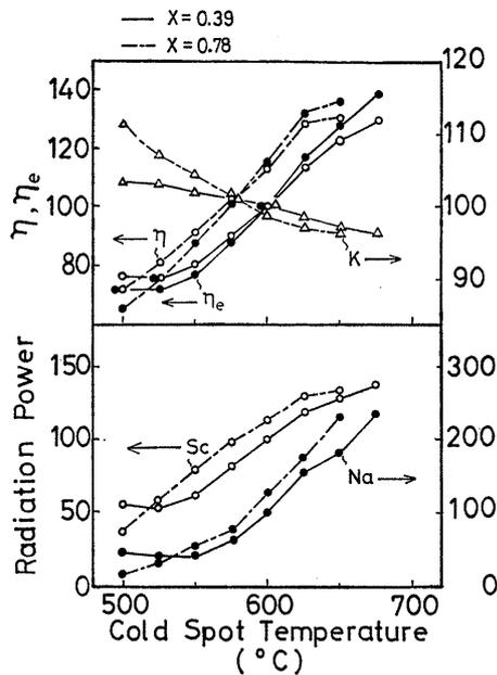
Fig. 5 Radiation properties with different mole functions as a function of the cold spot temperature.
