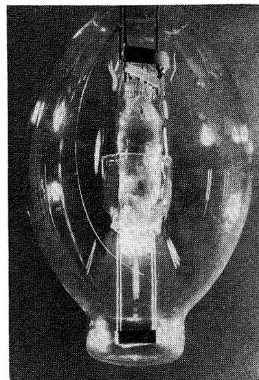
Fig. 8 A photograph of the lamp with a heat conserver.
