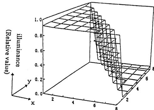
Fig. 11 Final illuminance on surface 1 (Kinoform is not installed)
