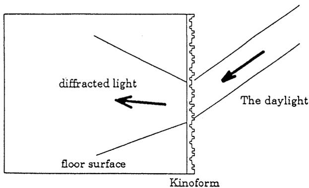
Fig.2(b) Conception of the propagation of the incident light
