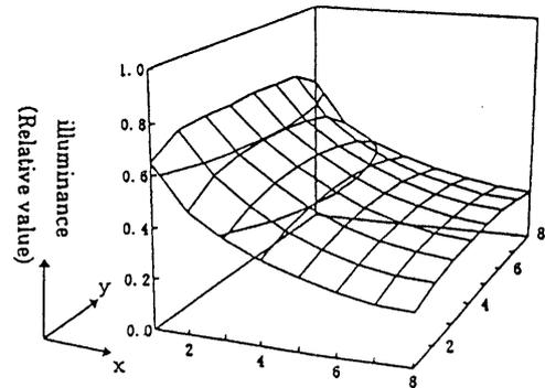
Fig. 10(b) Final illuminance on surface 1 (Boundary integral method, Method 2)
