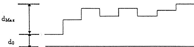
Fig.2(a) Cross section of kinoform
