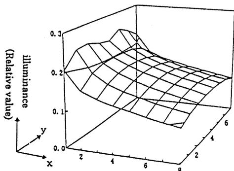
Fig. 10(a) Final illuminance on surface 1 (Boundary integral method, Method 1)
