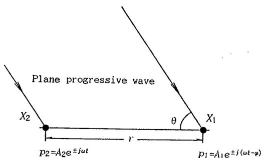
Fig. 1 Geometry of plane progressive wave and measuring points.
