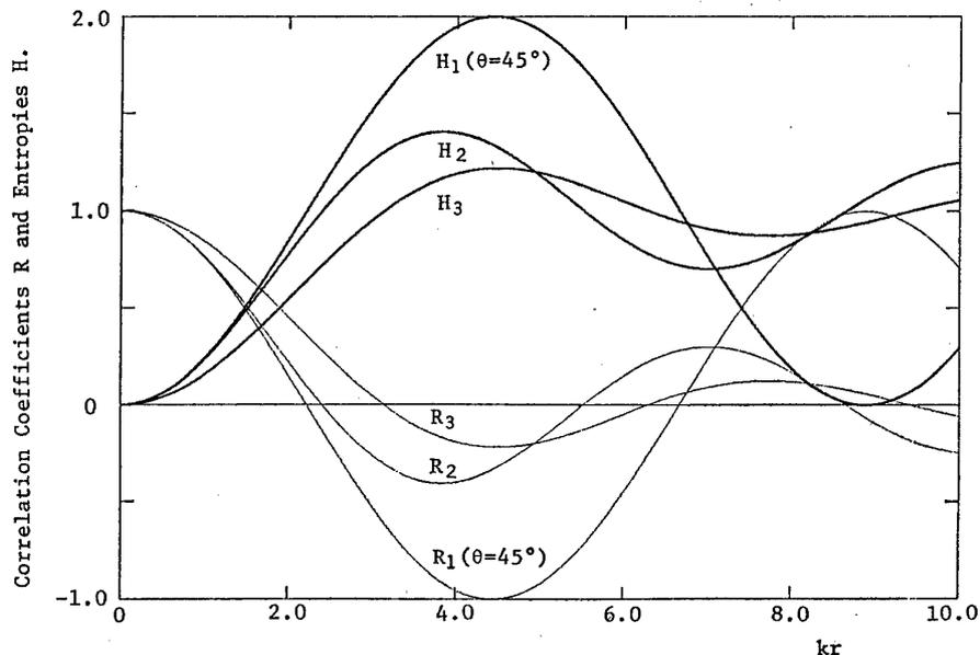
Fig. 2 Correlation coefficient and entropy in three kinds of sound fields (real parts).
