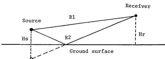
Fig. 1 The geometry of the source, the receiver and the ground surface.
