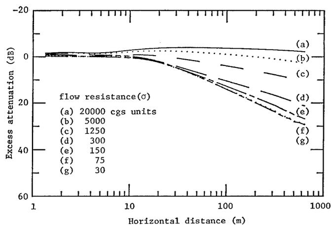
**Fig. 4** Comparison of A-weighted excess attenuation for various values of the surface flow resistance. The source and receiver heights are 0.3 m and 1.2 m respectively.
