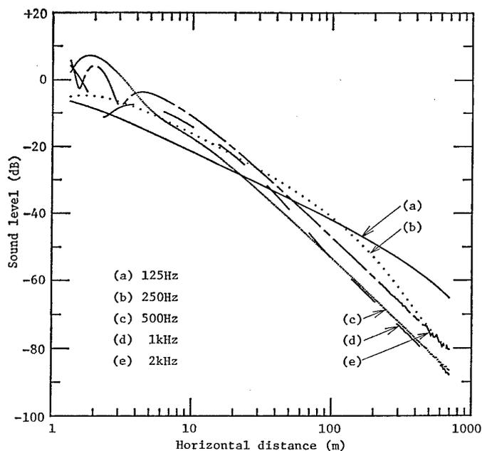
**Fig. 3** Comparison of sound levels calculated for octave band frequency components of A-weighted vehicle noise. The source and receiver heights are 0.3 m and 1.2 m above the ground respectively, and the ground resistivity is 300 cgs units.
