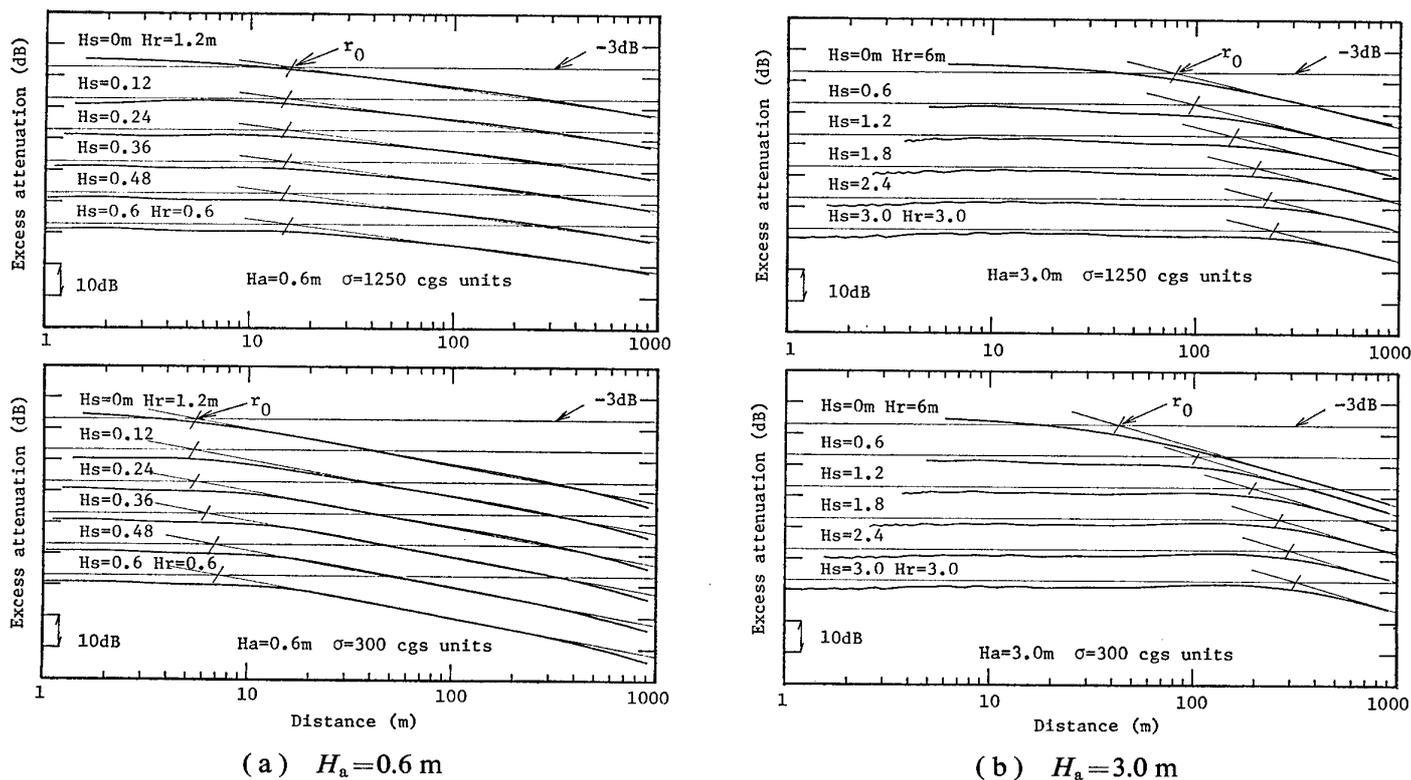
Fig. 5 A-weighted excess attenuation calculated under the condition of the same mean propagation height, i.e.,  $H_a$ , for three cases of  $\sigma = 1,250$  cgs units and  $\sigma = 300$  cgs units. The slant straight lines are the most suitable to each calculated values in the range from 10 m to 1,000 m. The locations of  $r_0$  are the cross points between the excess attenuation of  $-3$  dB and these lines.
