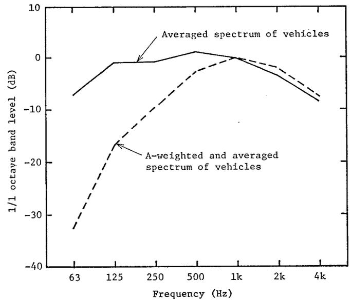
**Fig. 2** Typical 1/1 octave band spectrum (from Ref. 14)) of vehicles and A-weighted spectrum used to estimate the A-weighted excess attenuation.
