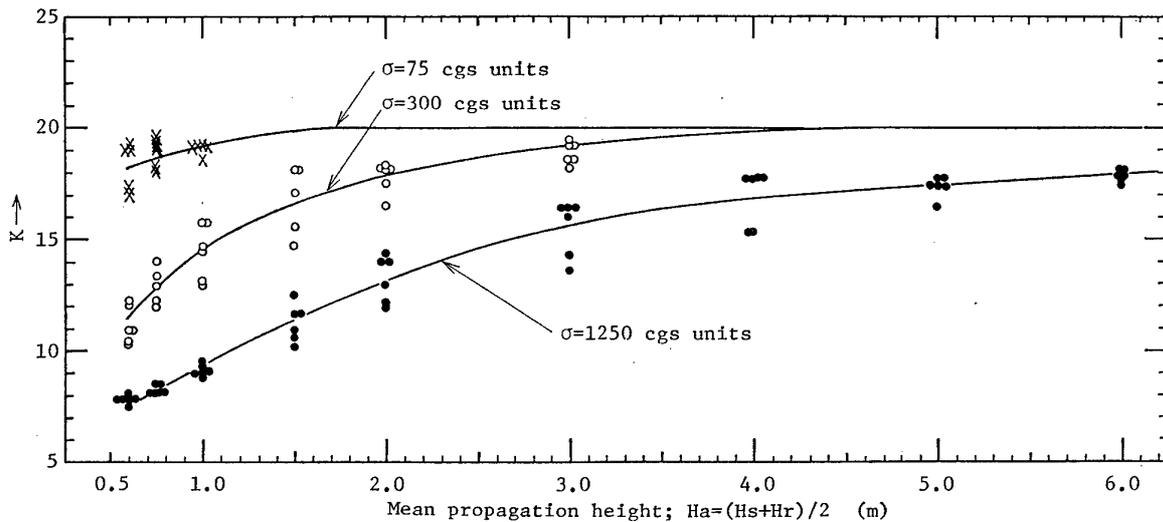
Fig. 6 The relationship between  $K$  and mean propagation height for three types of ground, i.e.,  $\sigma=75$  cgs units,  $\sigma=300$  cgs units and  $\sigma=1,250$  cgs units.
