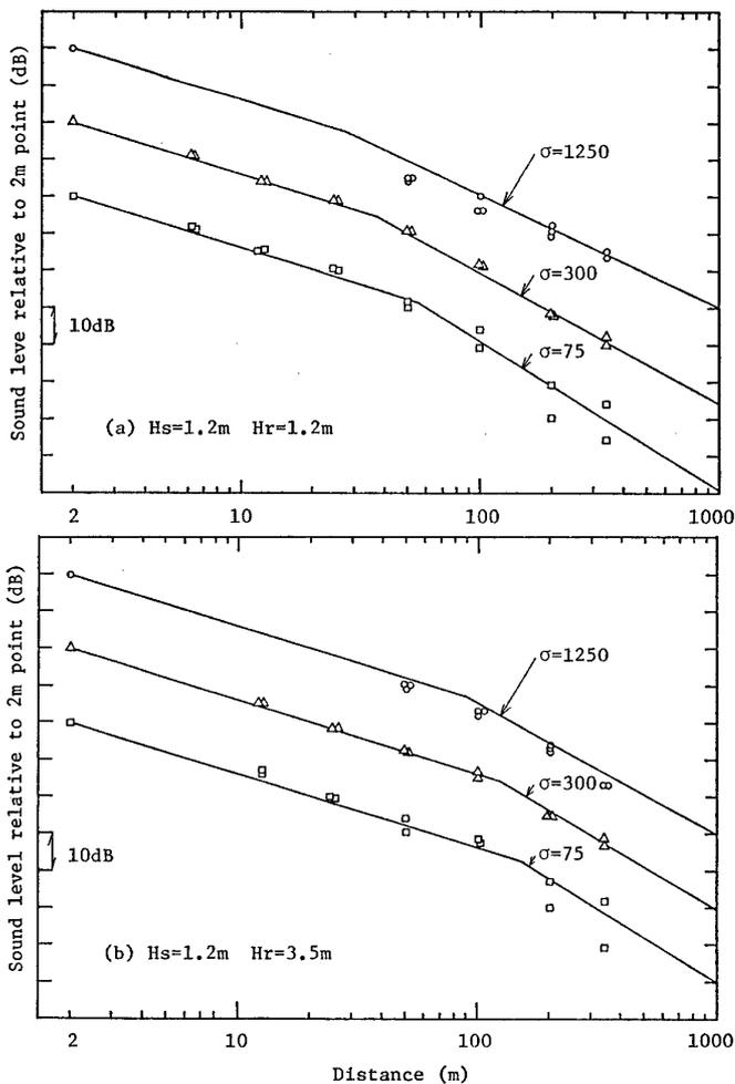
**Fig. 8** Comparison between the calculated values and the sound levels measured at three different conditions of ground surface, i.e., points  $\circ$  are at a rice field covered with short rice plants of 0.8 m height,  $\triangle$  at the same field just after the crops were reaped and  $\square$  at the field newly plowed. The source and receiver heights are respectively: (a)  $H_s=1.2$  m,  $H_r=1.2$  m; (b)  $H_s=1.2$  m,  $H_r=3.5$  m.
