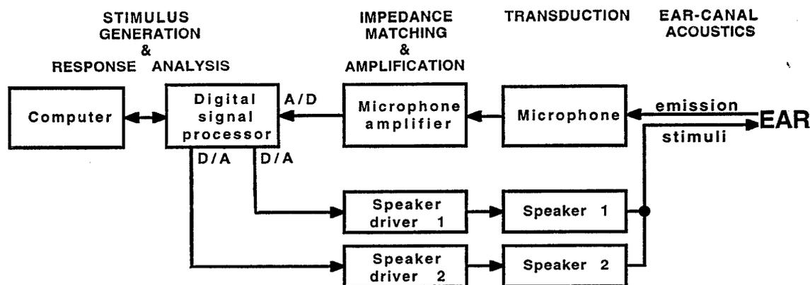
Fig. 1 Schematic of a typical equipment set-up for the measurement of OAEs. See text for explanation.
