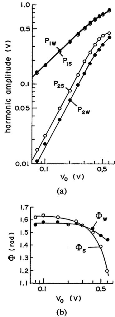
**Fig. 6** Influence of insertion of benzyl alcohol layer on received sound at various source levels. (a) Harmonic amplitudes. (b) Phase parameter.
