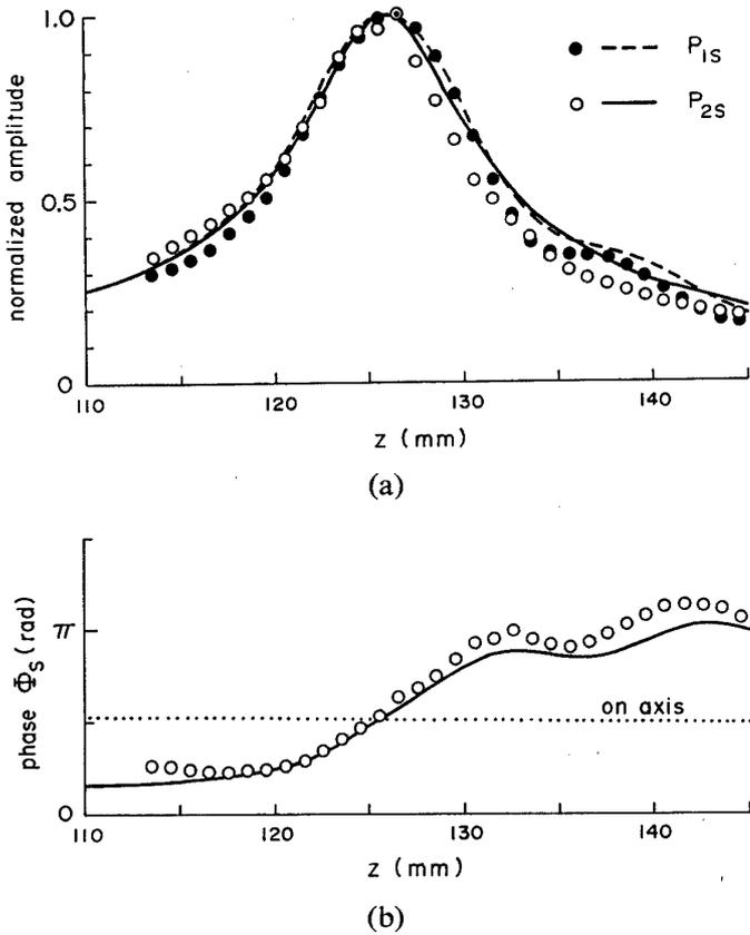
**Fig. 5** Range dependence of received sound with inserted sample layer. (a) Harmonic amplitudes. (b) Phase parameter.
