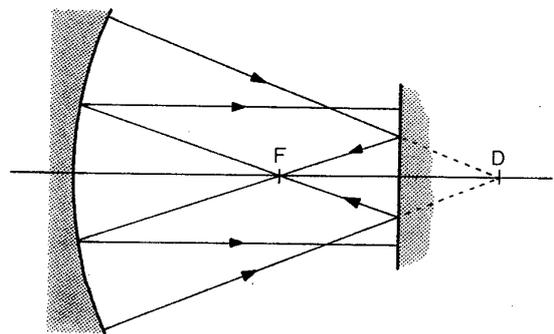
Fig. 4 Plane wave obtained with triple transition.<sup>16)</sup>
