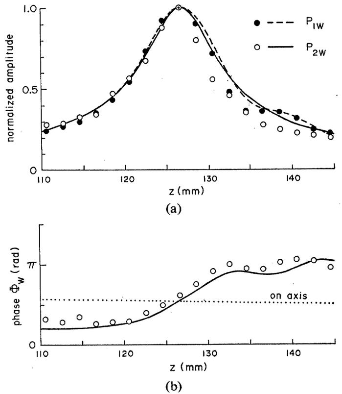
Fig. 2 Range dependence of received sound in free field. (a) Harmonic amplitudes. (b) Phase parameter.
