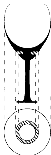
Fig. 7 Method for shaving a glass circumferentially.
