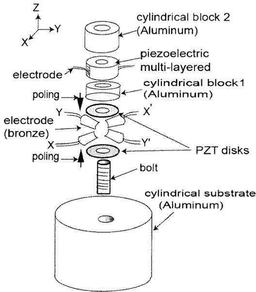
Fig. 1 Structure of the proposed multi-DOF motor.
