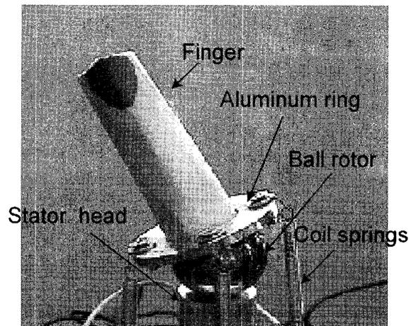
Fig. 5 Holding mechanism of the ball rotor.
