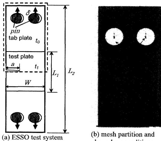
(a) ESSO test system (b) mesh partition and boundary conditions
