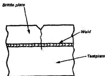
Figure 3 Duplex type wide plate test
