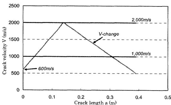
Figure 16 Crack velocity conditions assumed in FEM analysis
