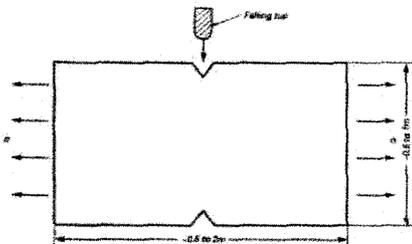
Figure 2 Principle and geometry of ESSO test
