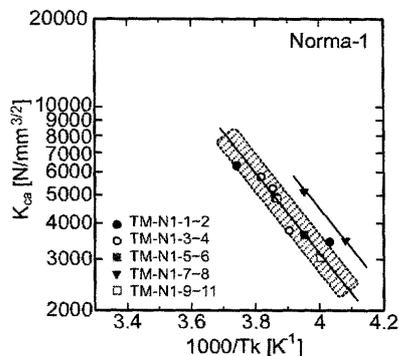
Figure 8 ESSO test result
