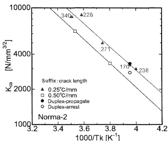
Figure 13 Effect of temperature gradient and crack length on  $K_{ca}$  evaluated by ESSO test (Norma-2)
