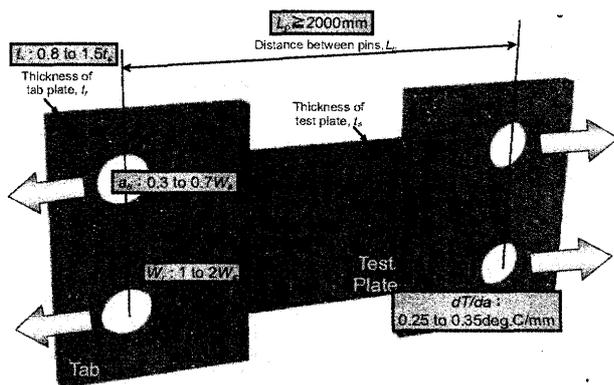
Figure 18 Major requirement in "BRITTLE CRACK ARREST TOUGHNESS  $K_{ca}$  TEST METHOD"
