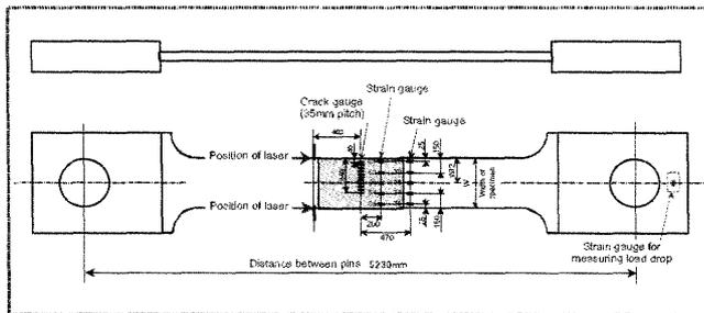
Figure 11 Dimension of specimen and tab plate and position of dynamic measurement (site B)
