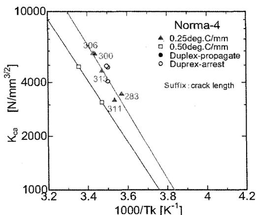
Figure 14 Effect of temperature gradient and crack length on  $K_{ca}$  evaluated by ESSO test (Norma-4)
