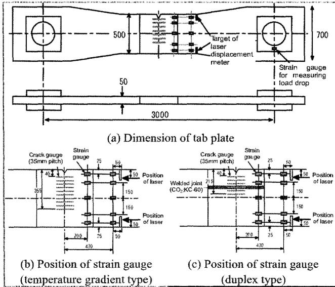
Figure 10 Dimension of specimen and tab plate and position of dynamic measurement (site A)
