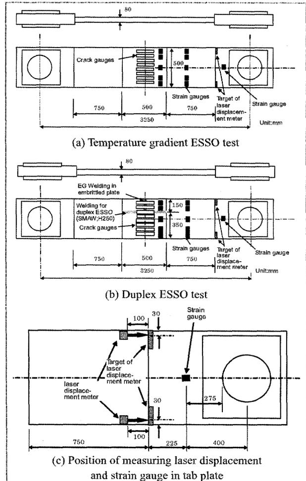
Figure 12 Dimension of specimen and tab plate and position of dynamic measurement (site C)
