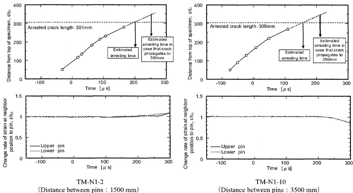
Figure 9 Breaking time of crack gauge and strain change around loading pin(TM-N1-2, TM-N1-11)
