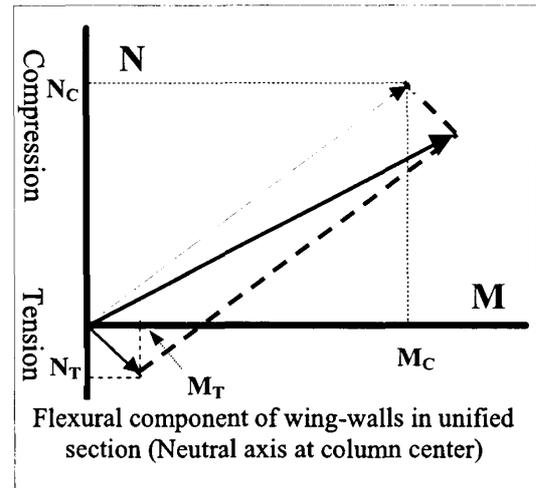
Fig. 6 Wing-wall flexural component
