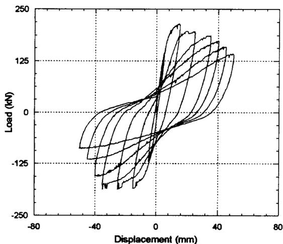
Fig. 10 Load-displacement curve for the specimen SJ-4
