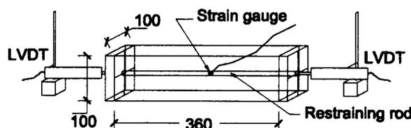
Fig. 2 Details of mould
