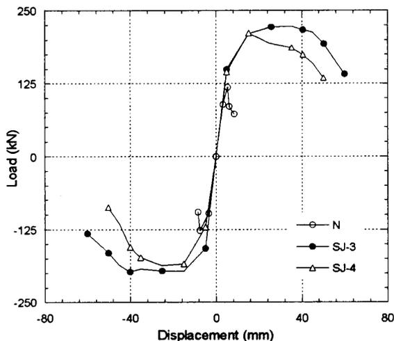
Fig. 12 Hysteresis envelope curves for the tested specimens
