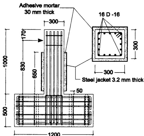
Fig. 1 Details of test specimen
