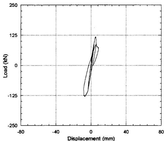
Fig. 7 Load-displacement curve for the control specimen
