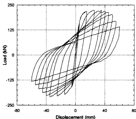
Fig. 8 Load-displacement curve for the specimen SJ-3
