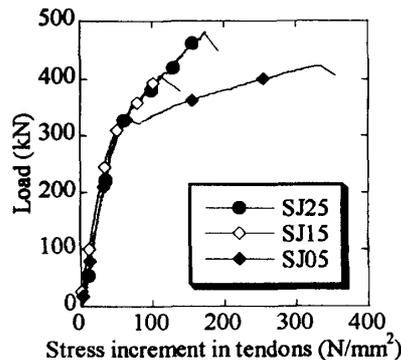
Fig. 7 Load-stress increment relationship
