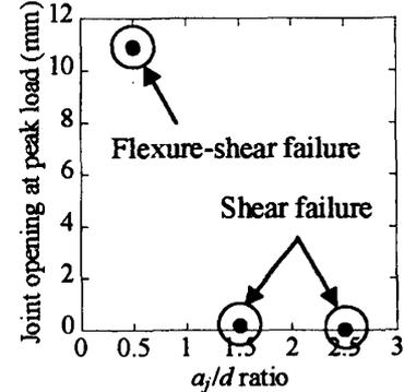
Fig. 11 Joint opening- $a/d$  ratio relationship
