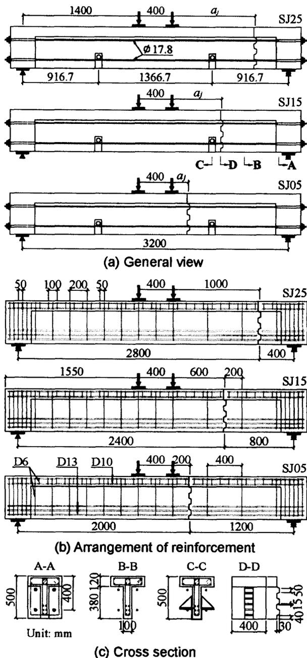
Fig. 1 Detail of test beams
