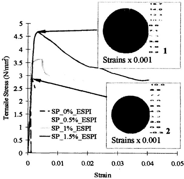
(a) Tensile strength and full field ultimate deformation pattern
