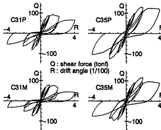
Fig. 5 Shear Force-Drift Angle Curves
