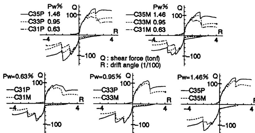
Fig. 6 Shear Force-Drift Angle Envelope Curves
