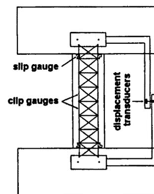
Fig. 3 Gauge Arrangement
