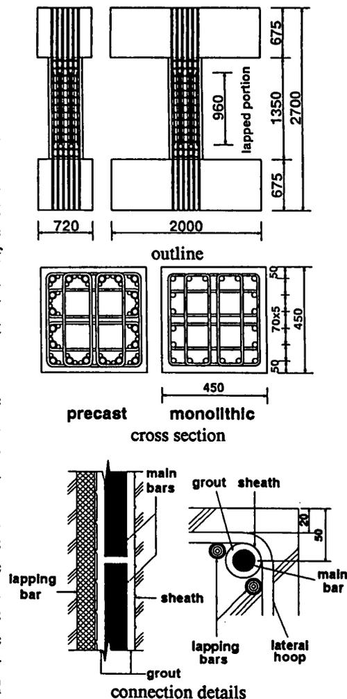
Fig. 1 Column Specimen
