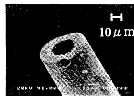
Fig.5 SEM image of Ti coated microneedle after wet etching.
