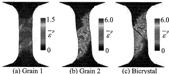
Fig. 5 Distribution of equivalent plastic strain
