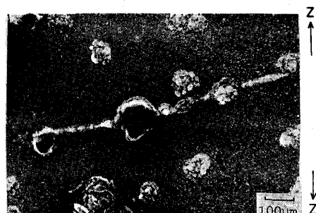
Fig.5 Corrosion groove initiated from a corrosion pit ( \sigma=35\text{MPa} ).
