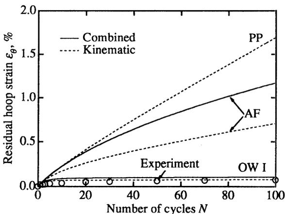
Fig.9. Increase of maximum residual hoop strain in 316FR steel cylinder subjected to axial travelling of temperature distribution [60].
