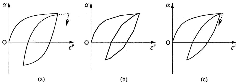
Fig.3. Change of uniaxial back stress  $\alpha$  under tensile straining followed by reverse straining and restraining.
