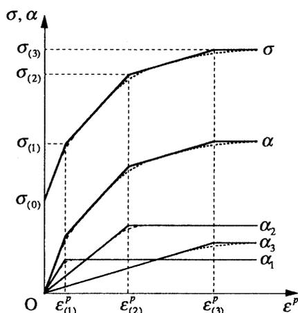
Fig.4. Changes of uniaxial tensile stress  $\sigma$  and back stress  $\alpha$ ; solid lines by Eq.(8) and dashed lines by Eqs.(10) and (11).
