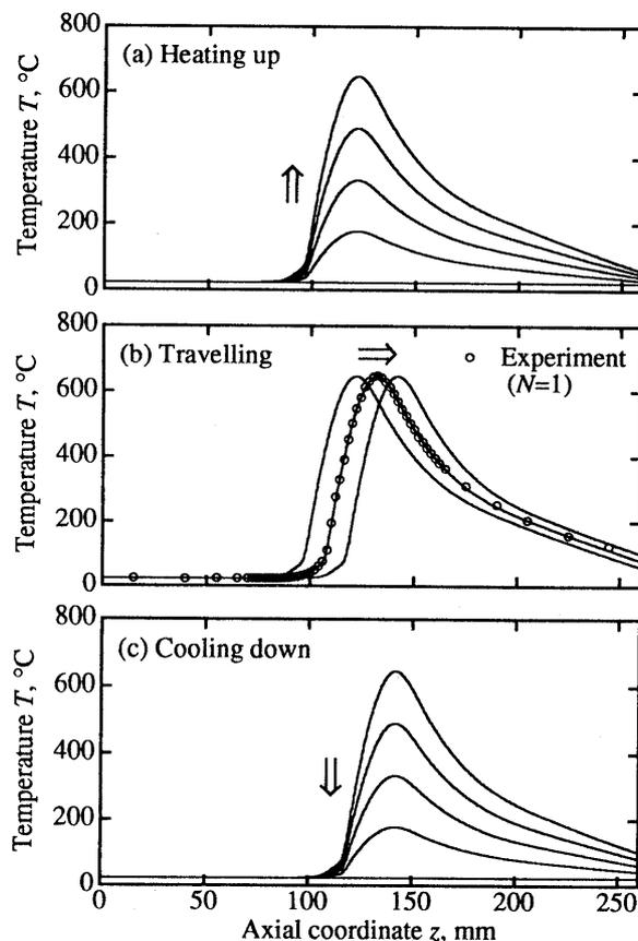
Fig.7. Thermal loading consisting of heating up, travelling of temperature distribution, and cooling down [1].
