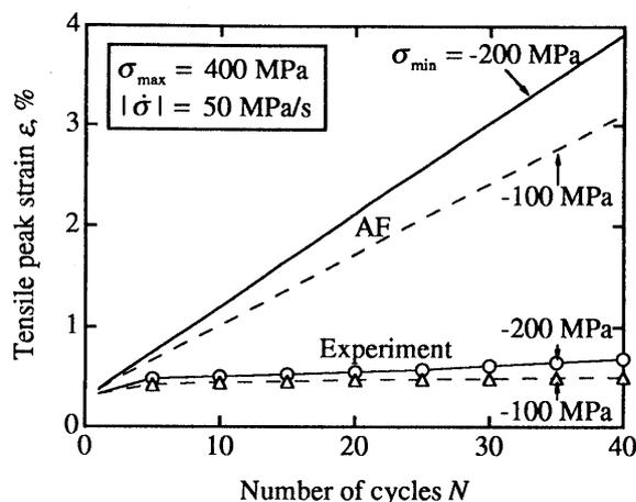
Fig.1. Uniaxial ratchetting of Modified 9Cr-1Mo steel at 550°C [28]; experiments [29] and simulations by the AF model.
