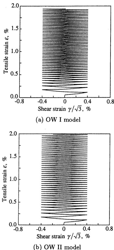
Fig.6. Application of the OW I and II models to the multiaxial ratchetting experiment shown in Fig.2(a) [28].
