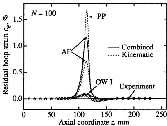
Fig.8. Distribution of residual hoop strain in 316FR cylinder after 100 cycles of axial travelling of temperature distribution [60].
