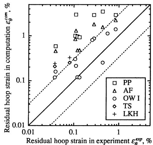
Fig.10. Comparison of experiments and computations with respect to maximum residual hoop strain in the last cycles in computation [2]; the models employed are PP (elastic-perfectly plastic), AF (Armstrong and Frederick), OW I (first version of Ohno and Wang), TS (PNC two surface [63]), and LKH (linear kinematic hardening).
