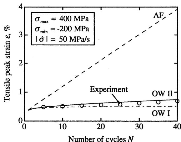
Fig.5. Uniaxial ratchetting of Modified 9Cr-1Mo steel at 550°C [28]; experiment [29] and simulations by the AF, OW I and OW II models.
