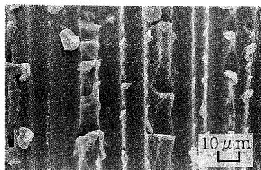
Fig.2. Fracture surface of 0° unidirectional composites (Kevlar49 composite. Dry-RT).
