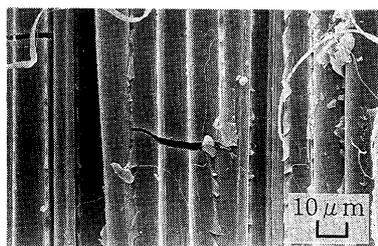
Fig.3. Fracture surface of 0° unidirectional composites (Kevlar49 composite. Dry-77K).
