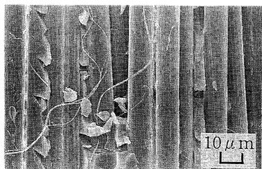
Fig.4. Fracture surface of 0° unidirectional composites (Kevlar49 composite. Wet-RT).
