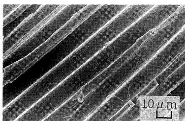
Fig.12. Fracture surface of  $\pm 45^\circ$  cross-ply composites (Kevlar49 composite. Wet-RT).
