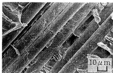
Fig.11. Fracture surface of  $\pm 45^\circ$  cross-ply composites (HM50 composite. Wet-RT).
