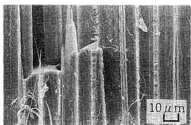
Fig.5. Fracture surface of 0° unidirectional composites (HM50 composite. Wet-77K).
