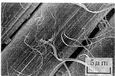
Fig.14. Fracture surface of  $\pm 45^\circ$  cross-ply composites (Kevlar49 composite. Wet-77K).
