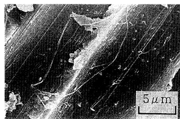
Fig.9. Fracture surface of  $\pm 45^\circ$  cross-ply composites (HM50 composite. Dry-RT).
