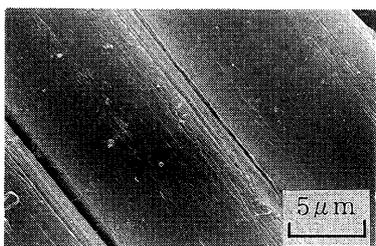
Fig.13. Fracture surface of  $\pm 45^\circ$  cross-ply composites (HM50 composite. Wet-77K).
