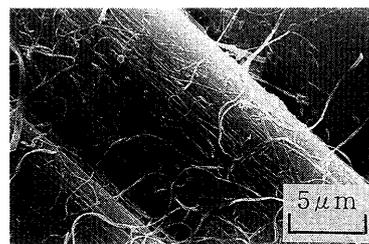
Fig.10. Fracture surface of  $\pm 45^\circ$  cross-ply composites (HM50 composite. Dry-77K).
