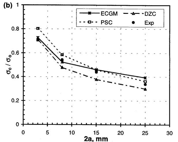
Fig. 5. Effect of notch size on residual strength (a) laminate A<sub>1</sub> and (b) laminate J<sub>1</sub>.
