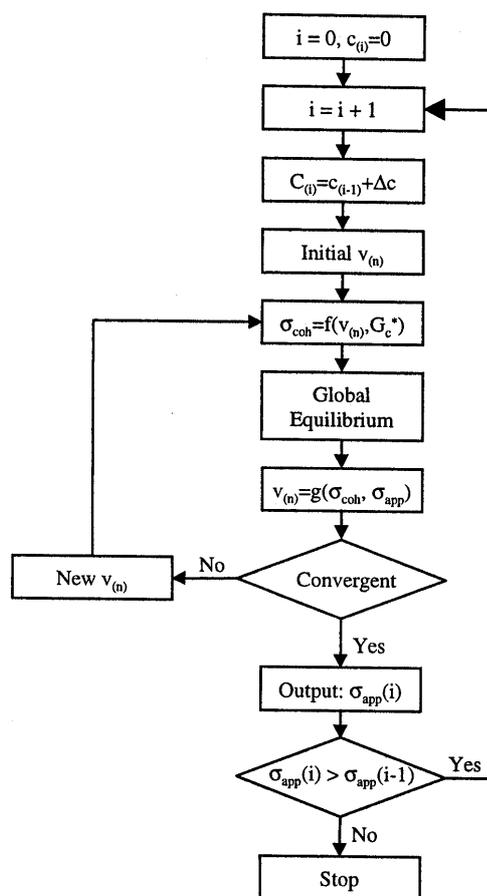
Fig. 2. Flow chart for residual strength evaluation by the ECGM.
