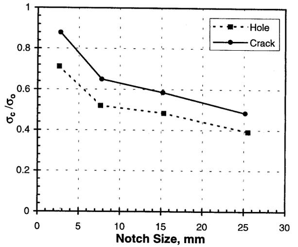
Fig. 4. Effect of notch shape on notch sensitivity of laminate K<sub>1</sub>.
