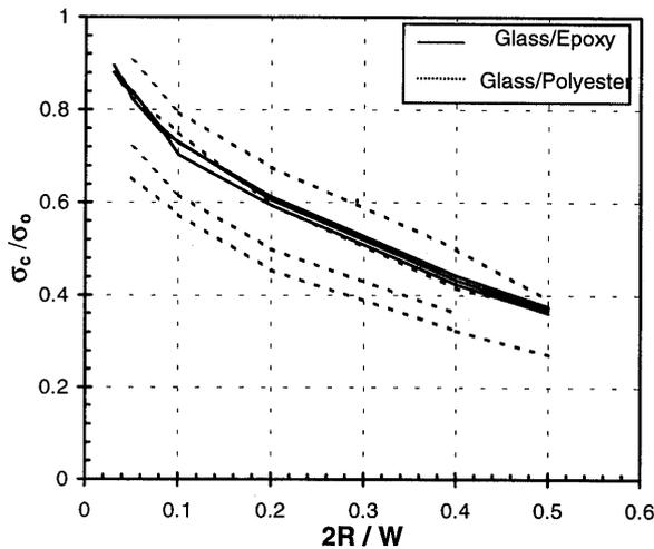
Fig. 3. Notch sensitivity of laminates D and E containing a circular hole.
