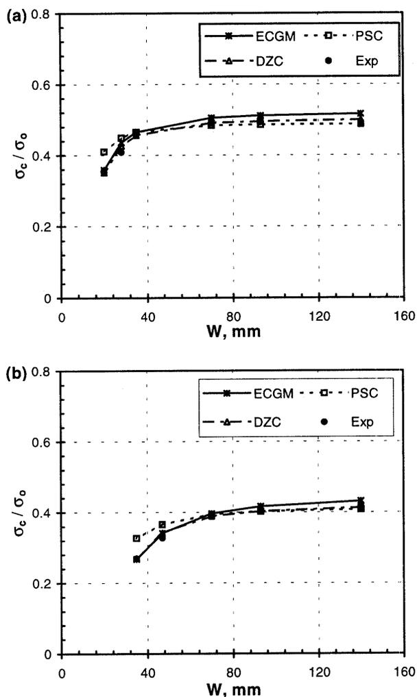
Fig. 6. Effect of specimen width on residual strength of laminate C (a)  $D = 10$  mm and (b)  $D = 20$  mm.
