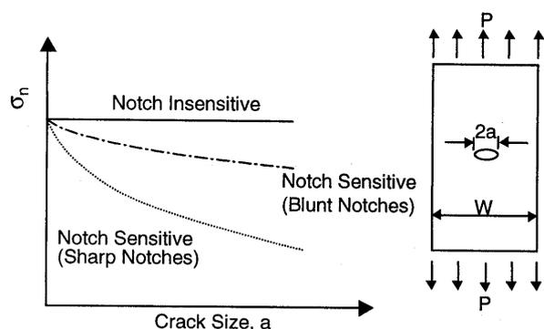
Fig. 1. Strength properties of notch sensitive and notch insensitive materials.
