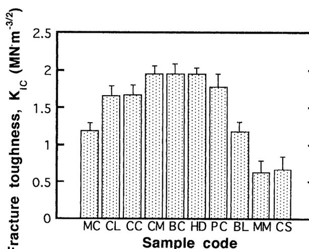
Fig. 2 Fracture toughness of eight core composite resins and two core cements.
