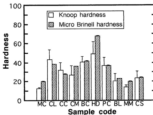
Fig. 3 Knoop hardness, Hk, and Micro Brinell hardness, MBH, of eight core composite resins and two core cements.
